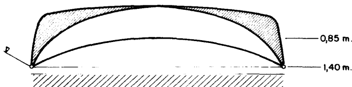
Fig.8.14: Diagram showing the shape of the groundwater table after recharge and during tail recession.
