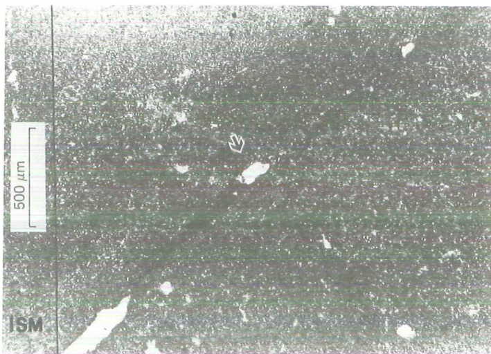
Fig. 13. Shear plane or slickenside in the soft calcic material of the 'striped' transition zone of Profile Arroyo 1 at a depth of 260 cm. The slickenside is visible as a dark line that connects several voids. The arrow indicates a quartz grain trapped in the shear plane. The photograph was taken in normal light. Photo courtesy ISM.
