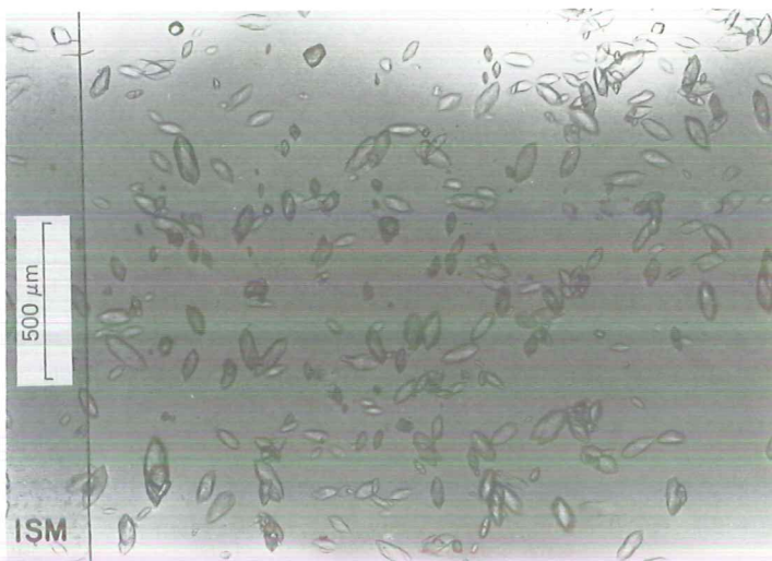
Fig. 15. Uniform silt-sized calcite crystals make up the material of the lime 'stripes' of Profile Arroyo 1 at a depth of 180 cm. The lime was loosely sprinkled into Canada balsam. The photograph was taken in normal light. Photo courtesy ISM.
