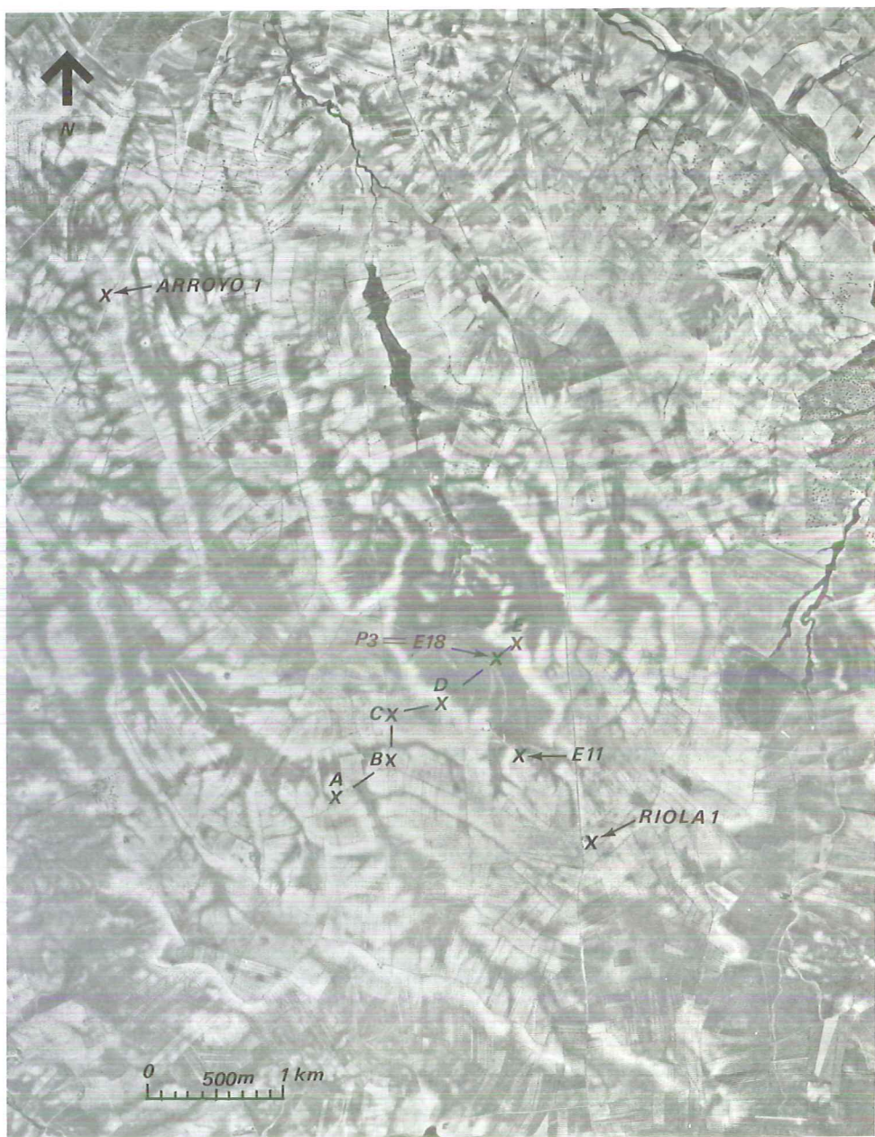
Fig. 4. Airphoto mosaic of the area south of Arroyo de San Servan in which most of the investigations were concentrated. The ridges and plateau edges which show up as light tones on the photo have petrocalcic horizons at or near the surface. The location of the three profiles of Section 4.3 and of the cross section AE has been indicated. Profile E11 of Fig. 41 is indicated too.
