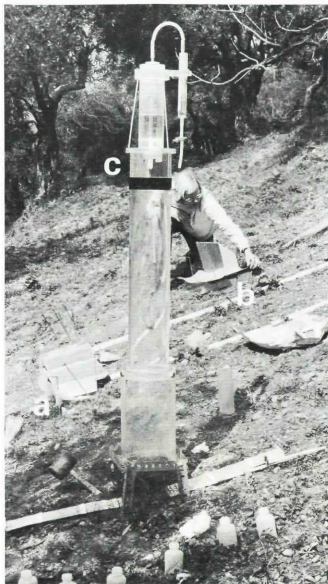
Plate 16 Field instrumentation on plot 11; a: the closed Gerlach throughs, measuring overland flow erosion; b: splash shields; c: portable rainfall simulator.
