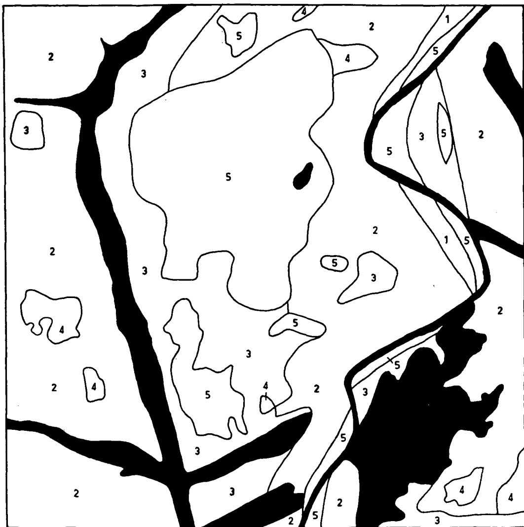
FIG. 144. Section of the map of present soil drainage conditions of the Hilla-Kifl project. 1. moderately well drained soils; 2. moderately to imperfectly drained soils; 3. imperfectly drained soils; 4. poorly drained soils; 5. very poorly drained soils; black: tel, argub, ruins.
