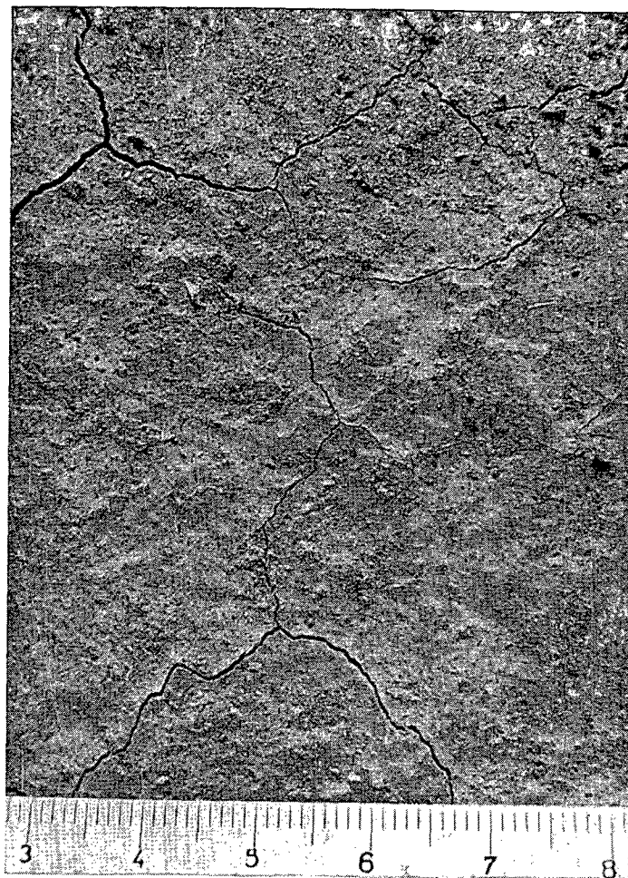
FIG. 59. Puddled and crusted surface layer of an irrigation levee soil. Almost all soils, which possess a layer of silty irrigation sediment on top have this hard non-porous crust (measure in cm.).
