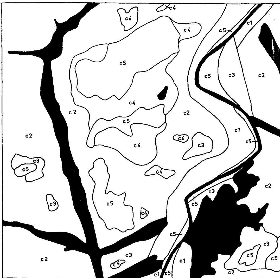
FIG. 147. Section of the potential soil suitability map for agricultural use of the Hilla-Kifl project. C1. excellent soils; C2. good soils; C3. fair soils; C4. poor soils; C5. very poor soils.
