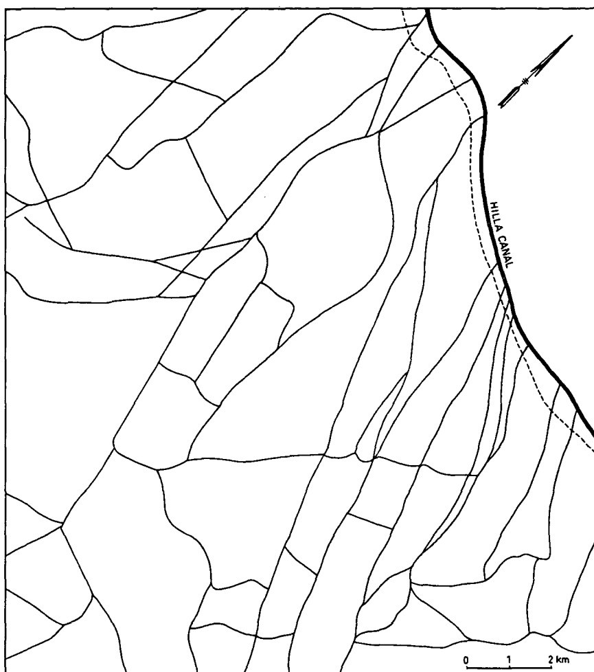
FIG. 73. Former system of controlled, canal irrigation in a large basin south of Babylon. In this way a large natural river basin is divided into numerous small irrigation basins, without drainage.
