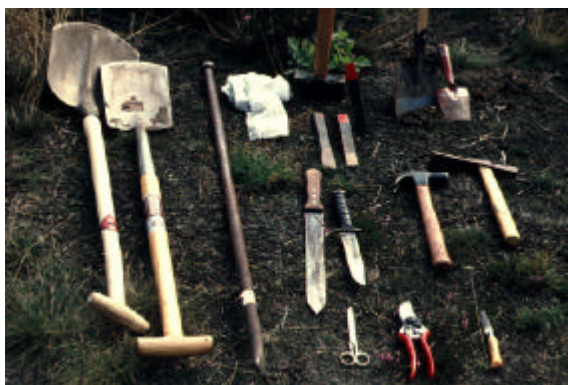
8. Field equipment for taking lacquer peels and soil monoliths
