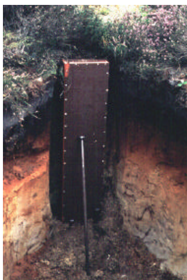
11. A box is pushed over the the column and held in position
