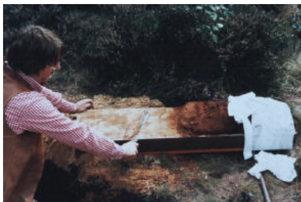
14. After removing the bandage, the profile is levelled
