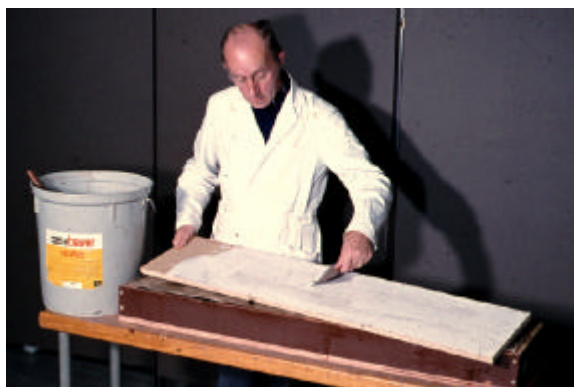
18. Chipboard is glued on the monolith
