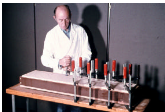
19. The chipboard is clamped onto the monolith
