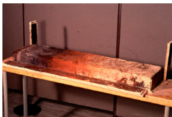
21. The box is removed from the monolith
