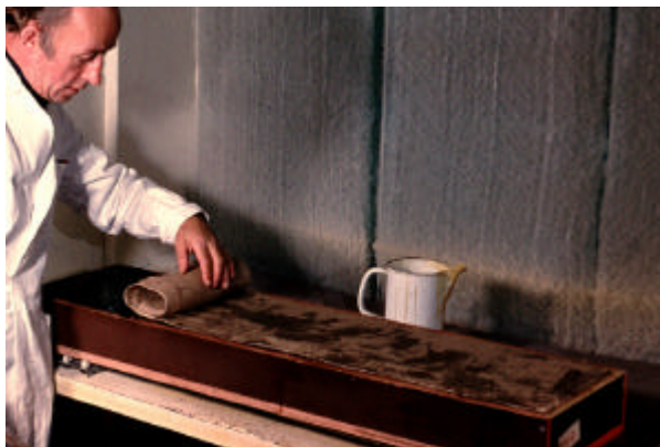
17. After drying, undiluted lacquer is applied, over which jute is applied
