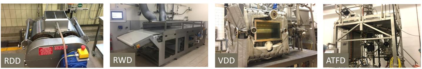
Refractance Window Dryer at ILVO Vacuum Drum Dryer at Andritz **Regular Drum Dryer at Unilever** Thesis Jun Qiu, FPE -WUR (2019) Systematic comparison of tomato powder quality prepared by four different conductive dryers.
