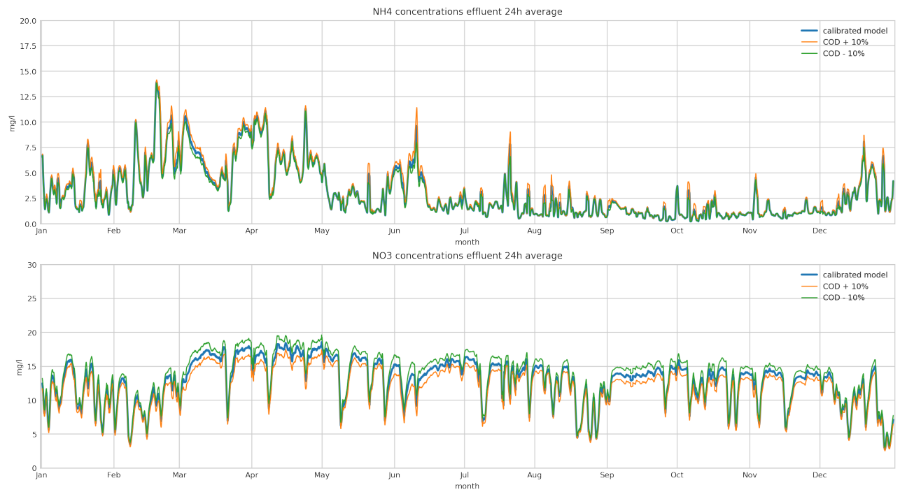
Figure 3.3.4: Variation in the effluent concentrations of ammonia and nitrate due to a 10% increase or decrease in the influent COD concentrations.
