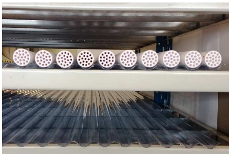
Figure 1: Pristine ceramic nanofiltration membranes in the laboratory of the Fraunhofer institute.
