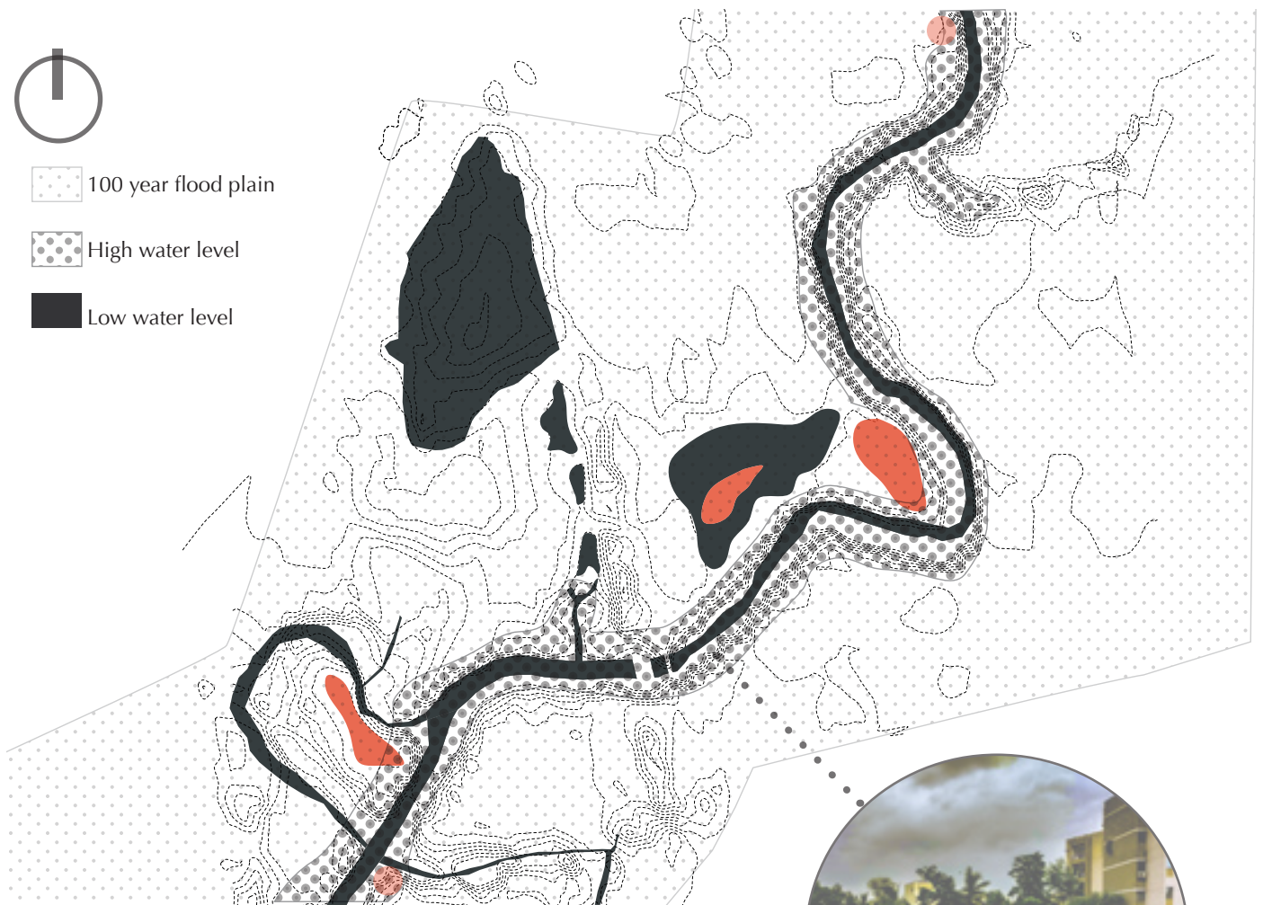
Fig. 55 The map below shows the locations for the mounds (on naturally raised areas) and the constructed wetlands (on naturally low-lying areas) along the river. The green dots indicate known crocodile nesting locations
