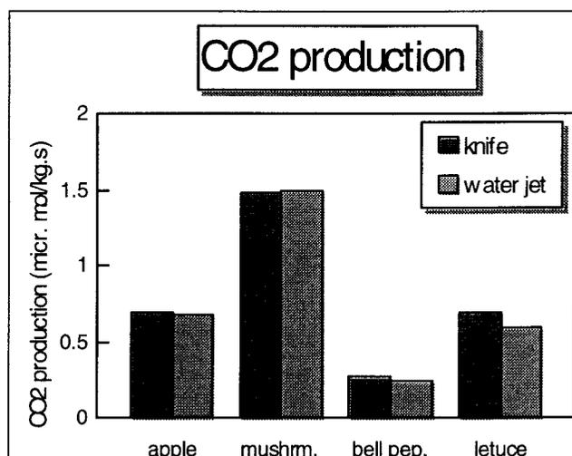
Fig. 20 Production of CO<sub>2</sub> of products with a knife and with a water jet.
