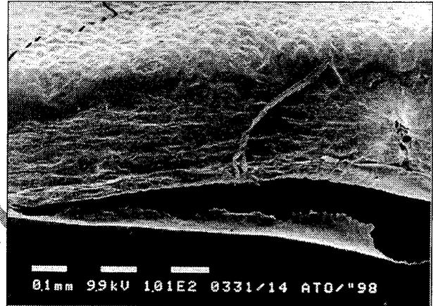
Fig. 13 SEM picture of lettuce, cut by the waterjet cutting system
