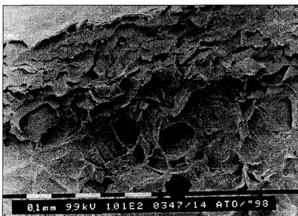
Fig. 17 SEM picture of red bell pepper, cut by the waterjet cutting system
