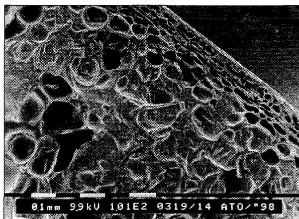
Fig. 11 SEM picture just under the peel of an apple strip, cut by the Urschel cutting system
