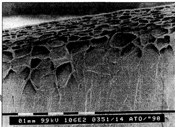
Fig. 18 SEM picture of red bell pepper, cut by the Urschel cutting system
