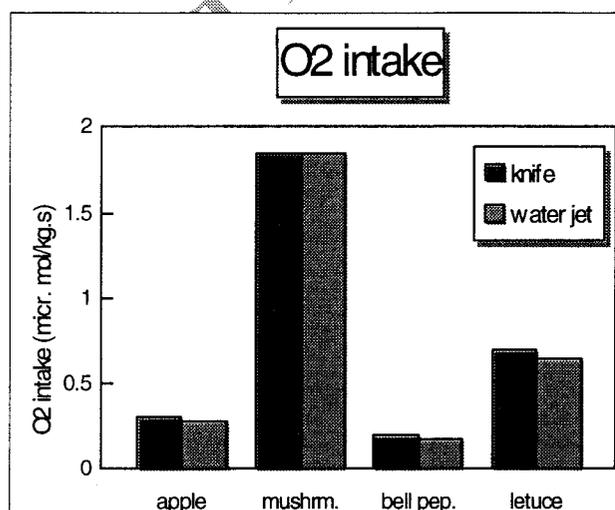
Fig. 19 Intake of O<sub>2</sub> of products cut with a knife device and with a water jet
