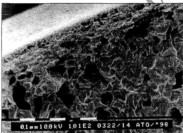
Fig. 10 SEM picture just under the peel of an apple strip, cut by the waterjet cutting system
