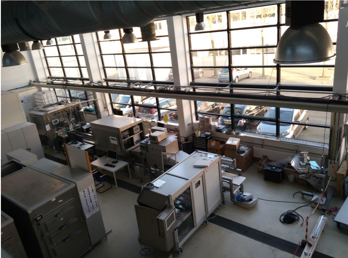
Figure 1: A global overview of Demo 1 of the integrated Pick&Pack line. The first module on the left is the thermoformer, though it is occluded in this image by the second module; the Marel pick and place robot. A sectional frame separates the Quality assessment module, including a X-ray scanner. At the end of the line the printer is located. Not that the Laser module (Demo 2) and Cable robot (Demo 3) are missing. These modules will be demonstrated separately, though there is still a reasonable perspective that they can be integrated with Demo 1 in time.
