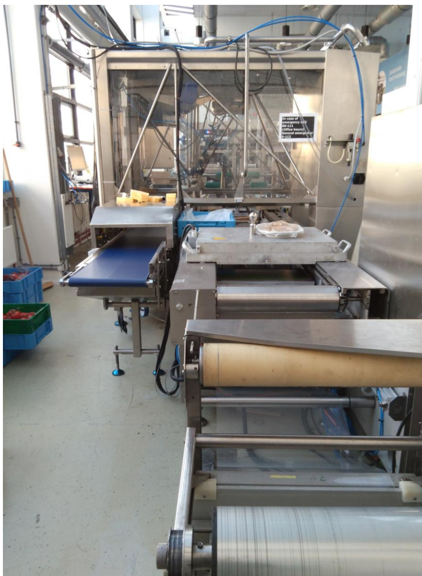
Figure 2: A side view from the beginning of the line; the thermoformer and the marel picking robot.
