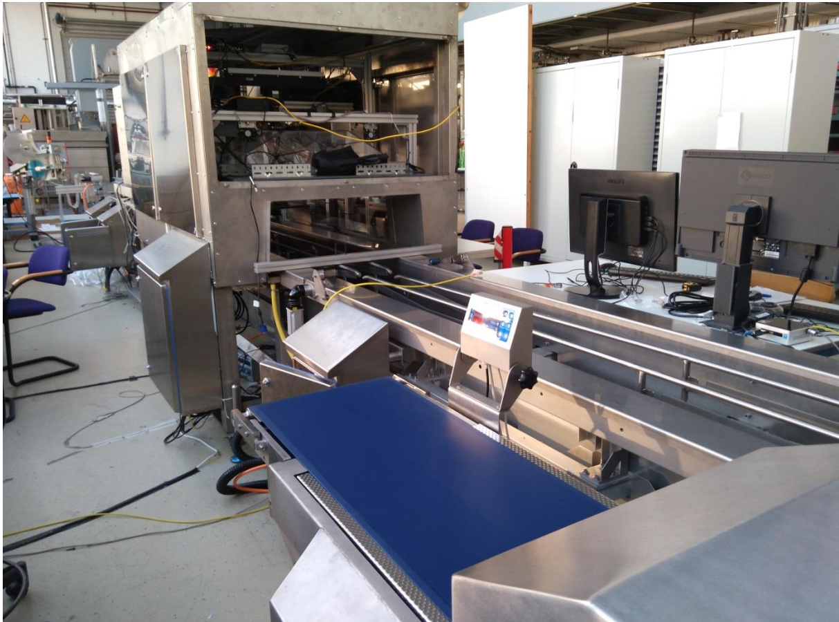
Figure 3: A side view from Demo 1; A sectional frame and the Quality Assessment Module. This sectional frame does not host a module and is intended to give an open view of the filled in packages. Optionally, it can be used for a dispensing unit or manual insertion of other food products.
