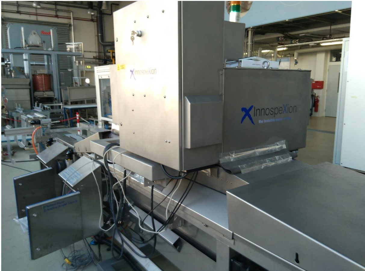
Figure 4: A side view from Demo 1; the QAS X-Ray device.
