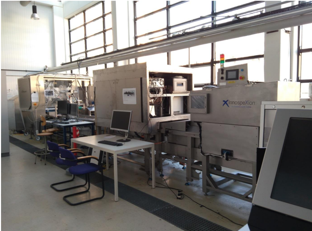
Figure 6: A side view of the integrated Demo 1 line. On the left the thermoformer and Marel robot. In the middle the QAS module and X-ray.
