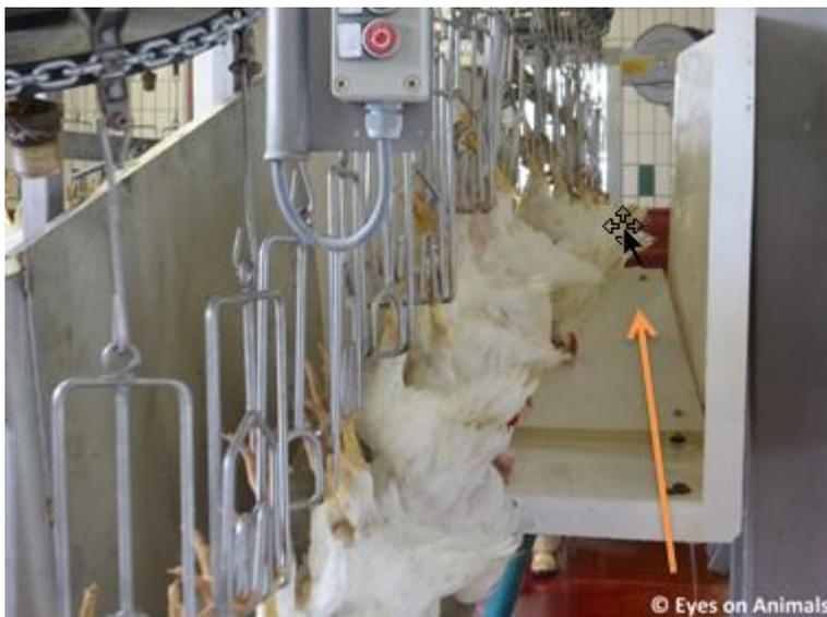
*Inclined ramp attached to the waterbath*
