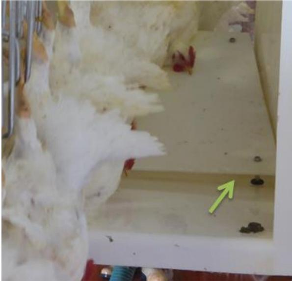
Space between inclined ramp and water bath stops water from getting on the ramp
