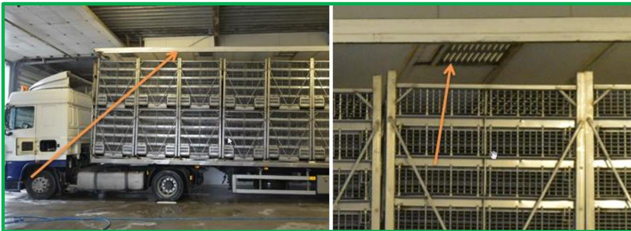
*Truck with roof that can be raised and air grills in the roof to let hot air out ©Eyes on Animals*
