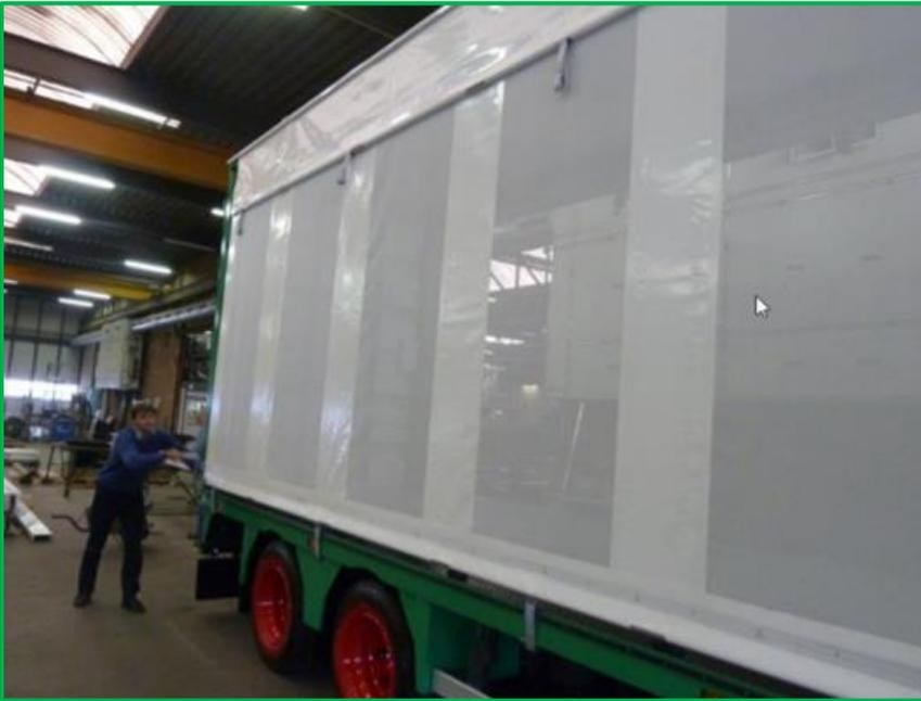
*Dual purpose tarp which can be quickly changed depending on the weather*
