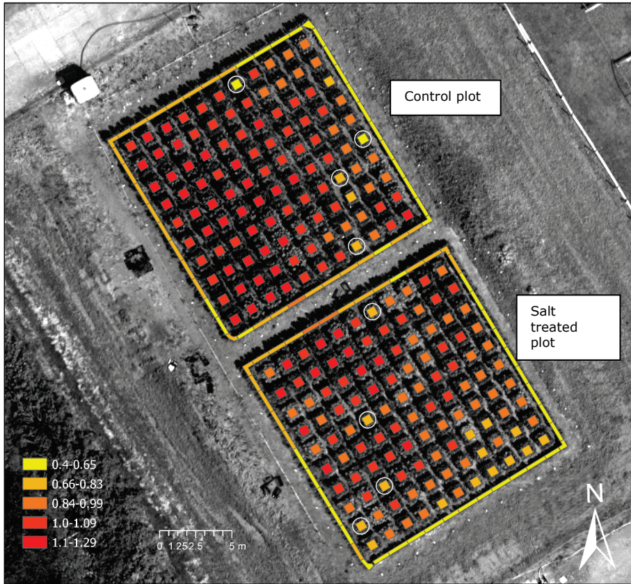
Figure 3.13. Lidar measured plant height (m) map (Pasto planting units are marked by the circles).
