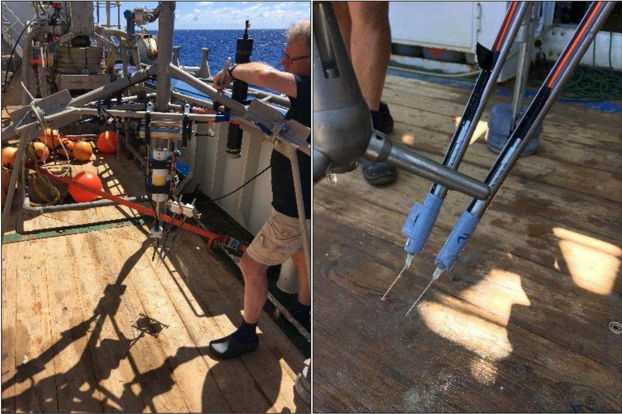
Figure 4.5.1. Left: Eddy correlation lander on deck; right: unisense oxygen microsensors bent after being hit by debris during a deployment
