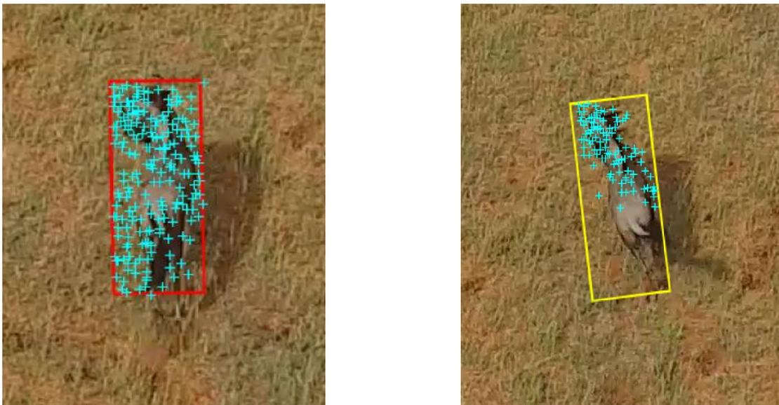
**Figure 2:** The feature windows calculated by the KLT tracking algorithm indicated as cyan dots in the initial frame (left) and in frame 10 (right). The red bounding box depicts the object of interest, selected by the user. The yellow bounding box represents the tracked object area.
