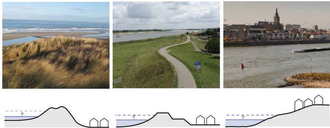
FIGURE 8.2 Photographs and diagrams of different elements of the Netherlands flood risk protection system a) natural sandy dunes, b) river dikes and c) natural high grounds. Photo of the natural high grounds of the city of Nijmegen by Rijkswaterstaat, Harry van Reeken.
