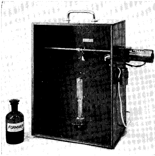
Fig. 16. Apparatus for preparing Formvar films on glass. (Designed by the Technical and Physical Engineering Research Service, Wageningen.)
