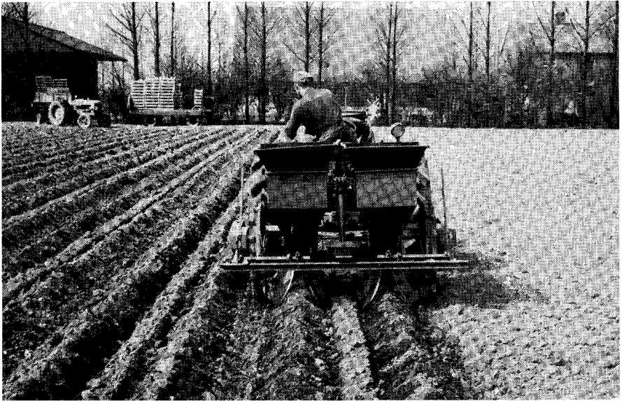
Fig. 60. Fully automatic planter. (From Institute of Agricultural Engineering and Rationalization, Wageningen.)
