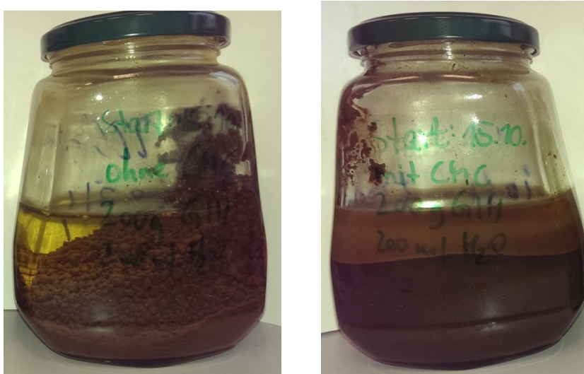
FIGURE 13: STABILITY OF PELLETS IN WATER. LEFT PICTURE: WITHOUT CMC; RIGHT PICTURE: WITH CMC.
