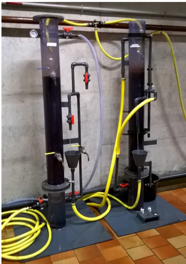
FIGURE 30 PILOT COLUMNS FILLED WITH GIH-PELLETS AT PRINSENBOSCH.
