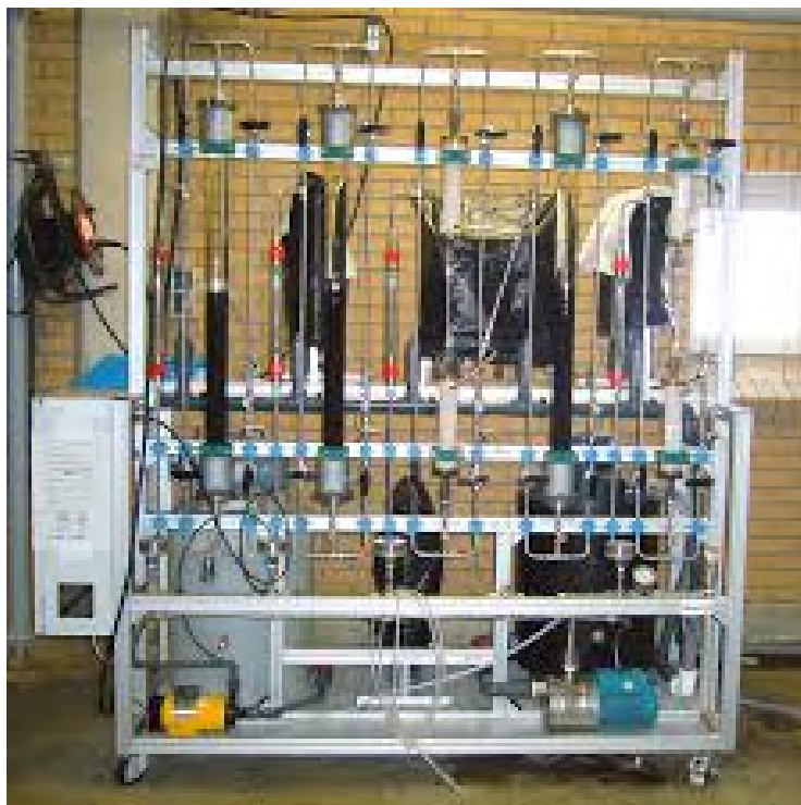
FIGURE 29 PILOT SETUP USED FOR ADSORPTION EXPERIMENTS AT KATWIJK
