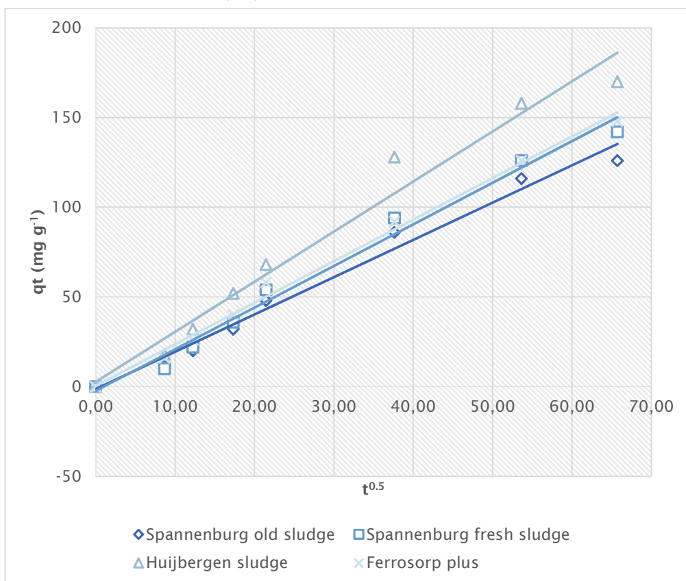
FIGURE 44 PLOT OF q_t AGAINST t^{0.5} . APPLICATION OF INTRA-PARTICLE DIFFUSION MODEL TO THE EXPERIMENTAL DATA OF FIGURE 7-1.
