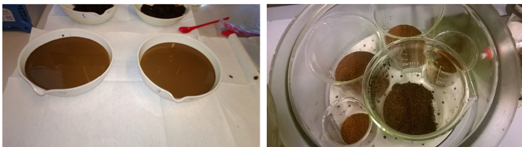
FIGURE 5 DRINKING WATER TREATMENT RESIDUALS BEFORE AND AFTER PROCESSING INTO PELLETS AT LABORATORY SCALE.
