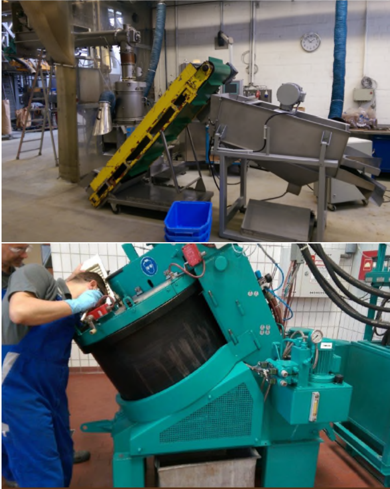
FIGURE 12: PELLET PRODUCTION AT AGRAVIS. UPPER FIGURE: EXTRUSION PROCESS, APPLYING PRESSURE. LOWER PICTURE: INTENSIVE MIXING PROCESS.
