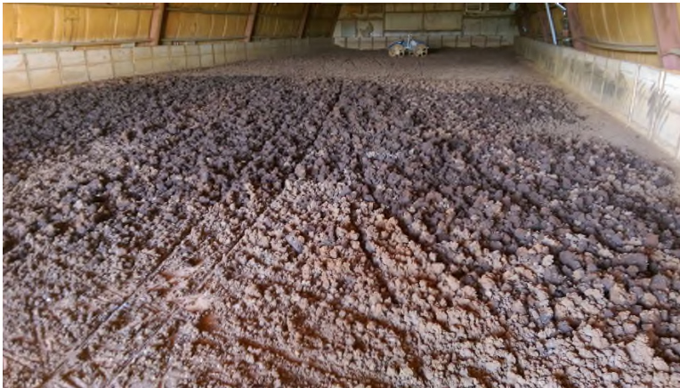
FIGURE 8 DRYING OF SPANNENBURG RESIDUAL BY MEANS OF WASTE HEAT FROM BIOGAS PLANT AND ELECTRIC MOLE.
