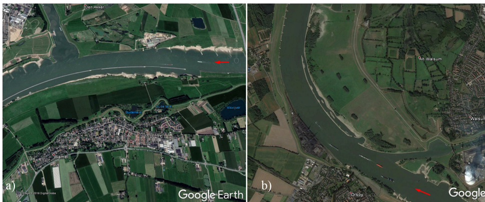
Figure 1.2: Examples of river training with longitudinal training wall a) near Wamel in The Netherlands, b) near Walsum-Stapp in Germany. Source: Google Earth © 2017.
