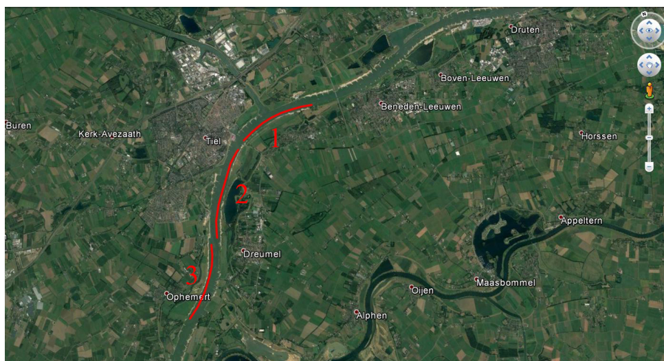
Figure 5.1: Three pilot LTDs on the Waal River (named 1, 2, and 3). Source: Google Earth © 2017. Flow direction from right to left. The red lines are the LTDs.
