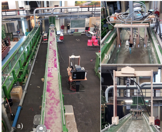
Figure 1.5: Flume used in this study and its components. a) General view with the formation of alternate bars; b) lasers devices to monitor bed and water level; c) high speed camera to monitor surface velocity.
