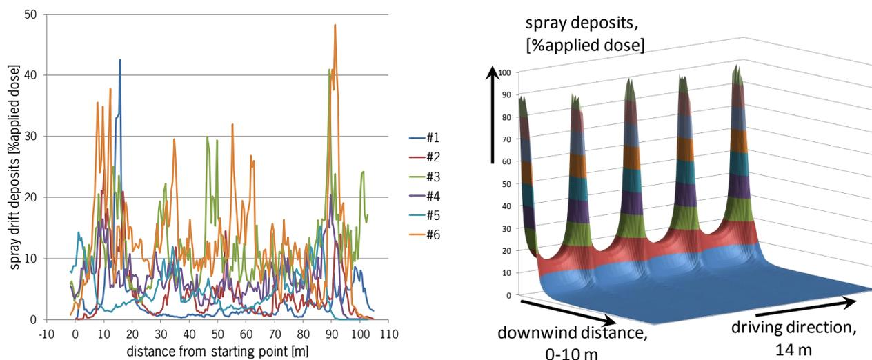
**Figure 2:** Left: measured spray drift deposits at 2 m downwind from the treated field, as a function of distance alongside the field; 6 repetitions are shown; right: simulated spray deposits downwind for sinusoidal horizontal sprayer boom movements at 0.50 Hz
