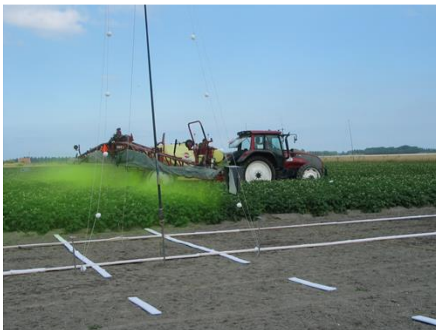
Fig. 1. Tractor and Hardi Commander sprayer driving through potato field, parallel to a bare soil field. Filter strips parallel to the field edge allow measuring variation in deposits along the edge.
