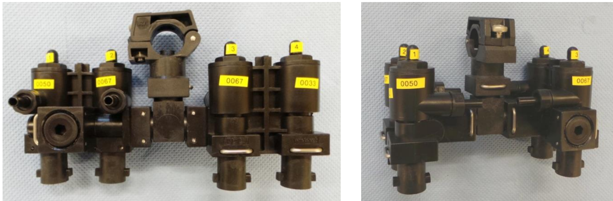
Fig. 2. Lechler varioselect fourfold block. Left : longitudinal configuration (L); right : square configuration (S). Nozzle positions are numbered (1..4), nozzle sizes are indicated for each position.
