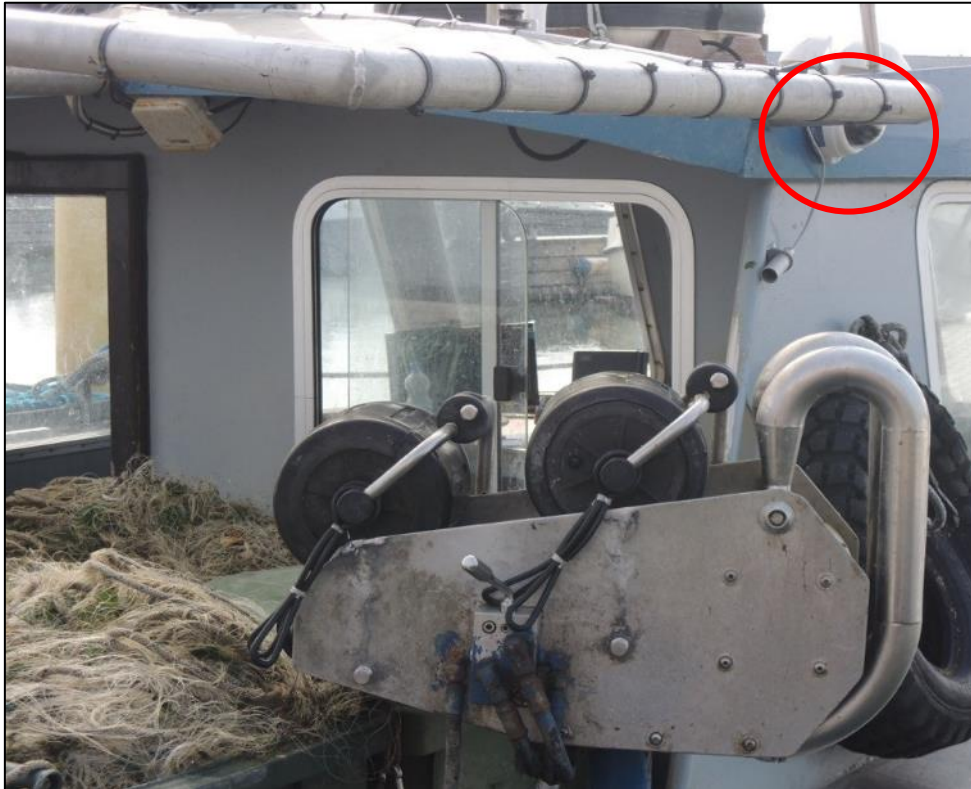
Figure 3. An example of the camera placement on board one of the participating vessel. The red circle shows the position of the camera [photographer: Marije Siemensma, MS&C].
