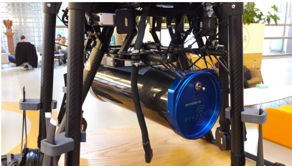
Figure 1: MS1000 gamma-ray spectrometer underneath a UAV
