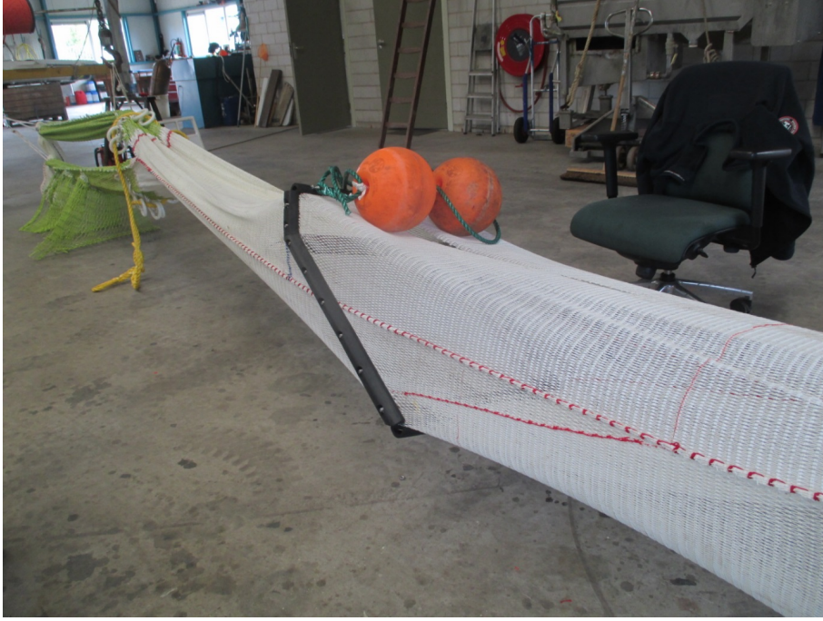
Figure 2: Single-grid gear under construction in the net loft. The oblique red selvedge is the connection of the guiding panel to the net tunnel.
