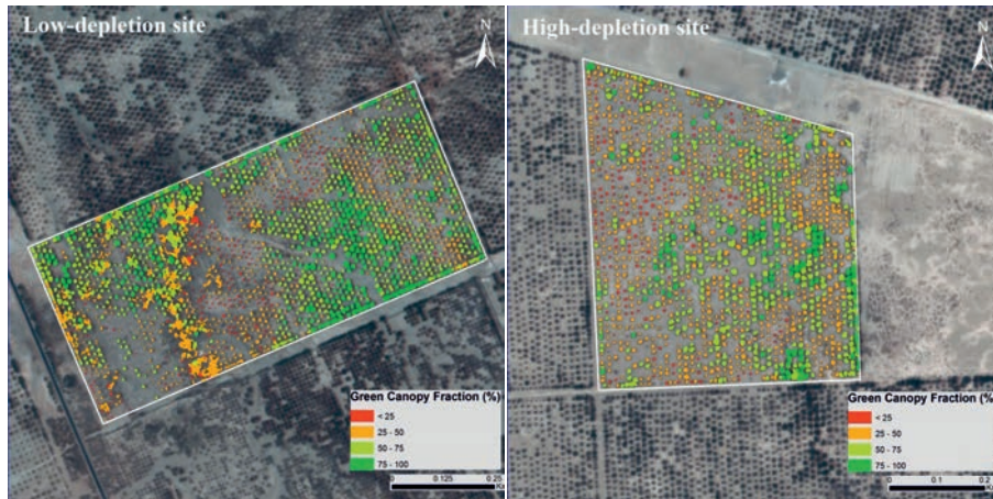
Figure 3.4: Green Canopy Fraction (GCF) derived from high-resolution (2.4 m pixel resolution) Worldview2 satellite data (acquired in July 2011).
