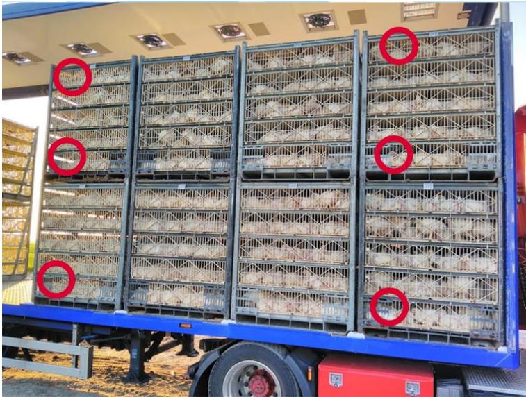
**Figure 21 Containers with thinned broilers, red circles indicate the place of the loggers at one side of the truck.**
