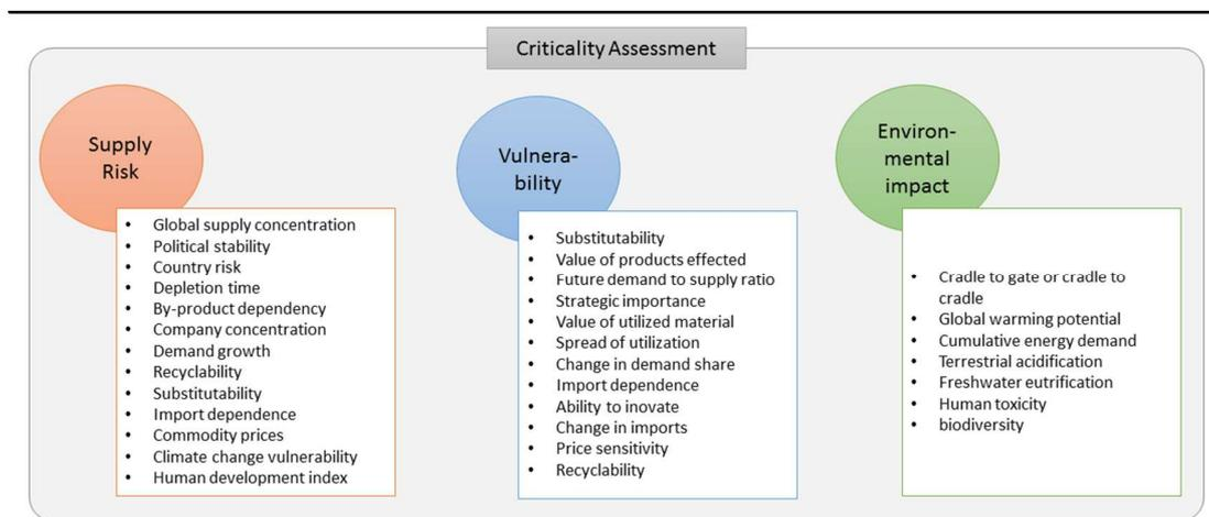
**Figure 2.1 Structure criticality assessment and possible indicators**
