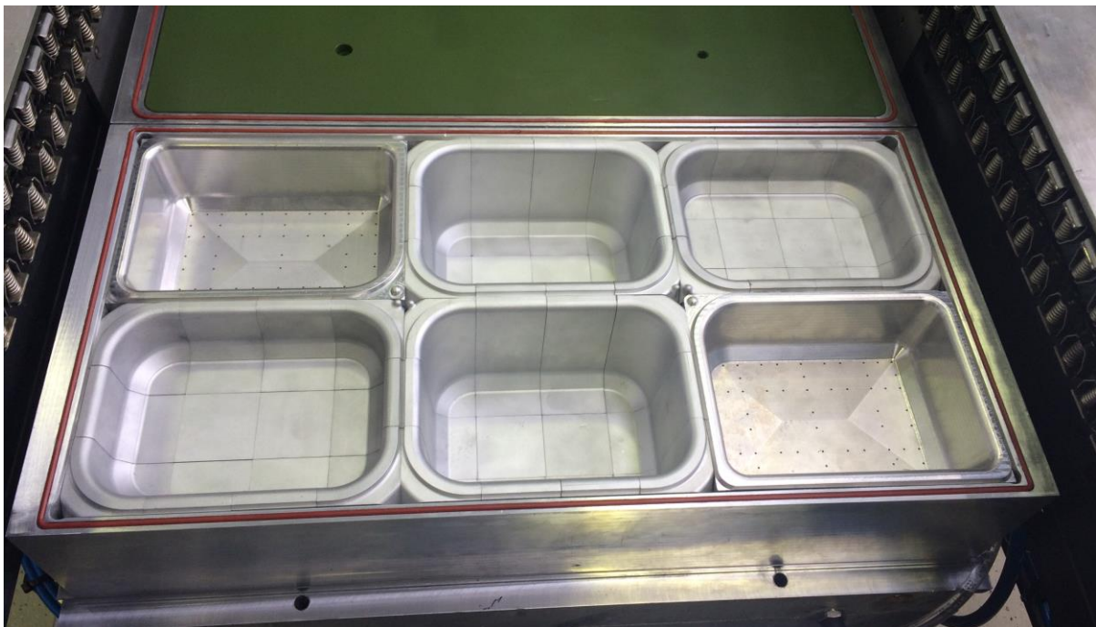
Figure 3 – Brick mould system installed in the thermoformer
