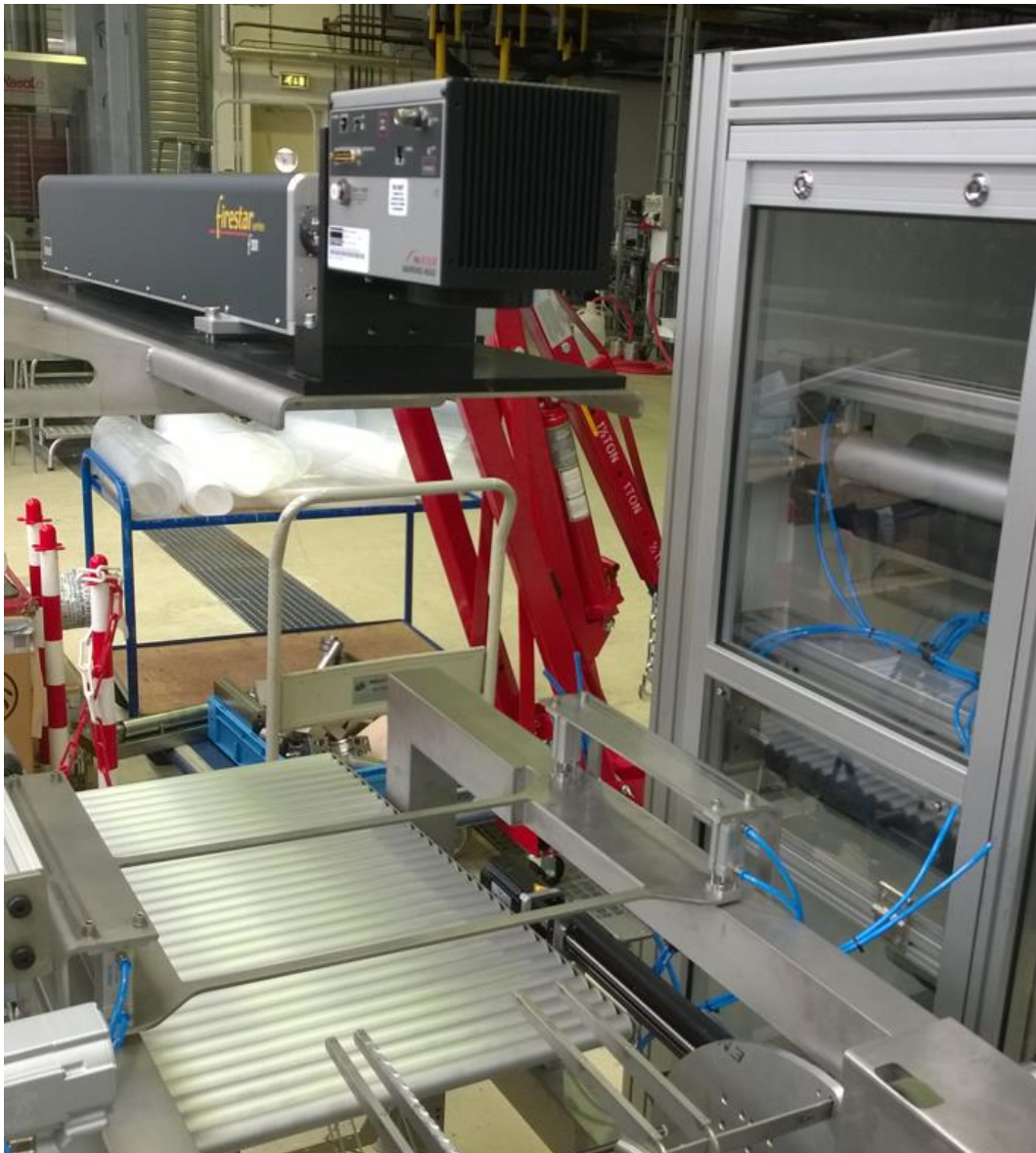
Figure 7 – Laser equipment on top, printer right and cross section.
