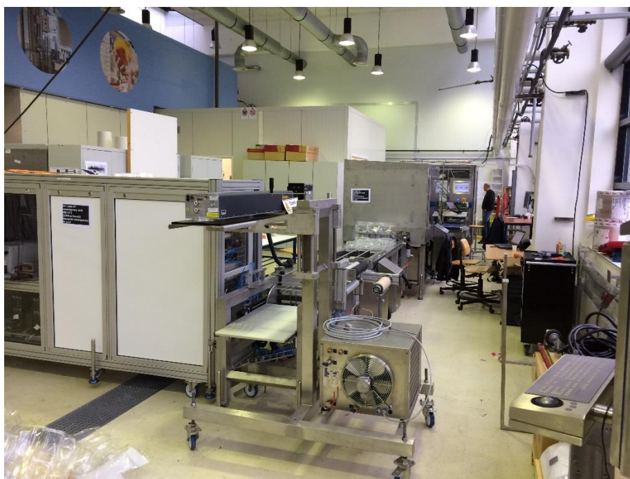
Figure 9 – Photo of the printer and laser for welding and cutting in Wageningen. Other modules as sectional frames, scanner and robot is also on the photo.
