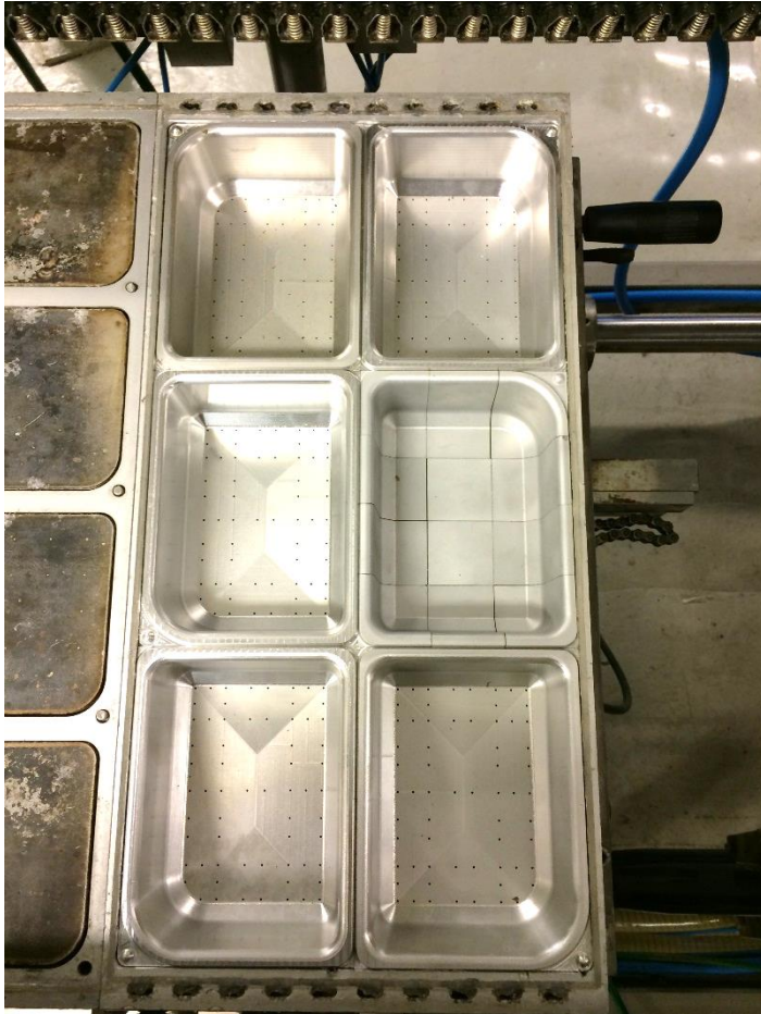
Figure 2 - Prototype of Brick Mould built into Vacuum Mould for the actual Thermoformer
