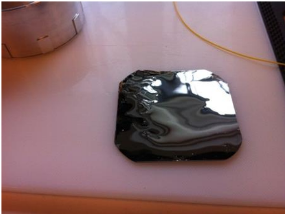
Figure 25 - The sample with the silver coating printed for 6 passes with 360 dpi resolution.
