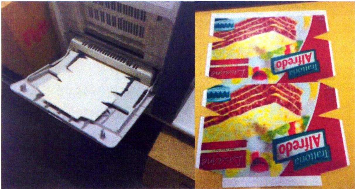
Figure 30 - Precut cardboard printed on ordinary office printer
