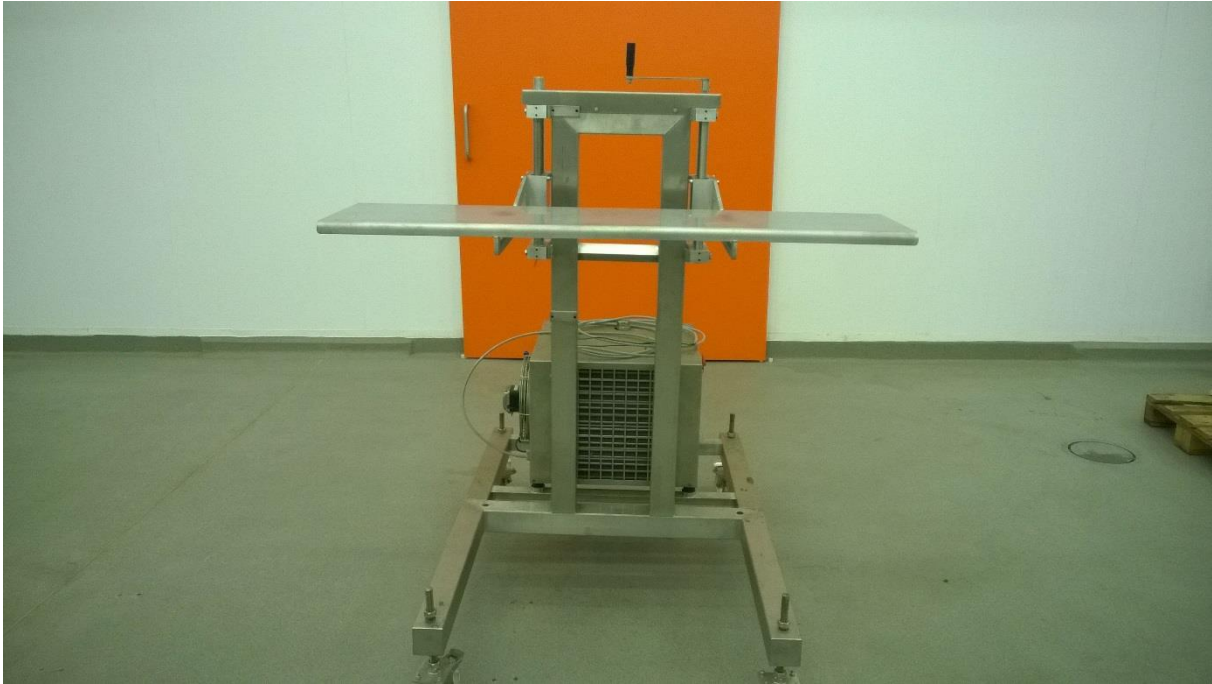
Figure 12 - Frame for laser to be used in PicknPack line. There will also be built screens around the laser marking head
