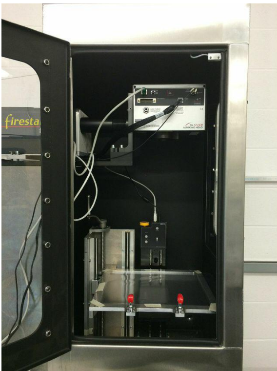
Figure 11 - A view into the laser marking head and a sample of the foil to be sealed
