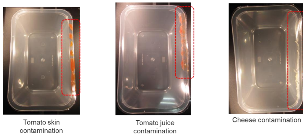
Figure 19 - Contamination of seals with tomato skin (left), tomato juice (middle) and cheese (right). For each package, only one half was contaminated.
