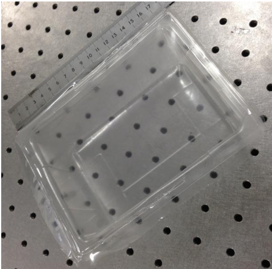
Figure 15 – Tray made in the brick mould that is laser welded
