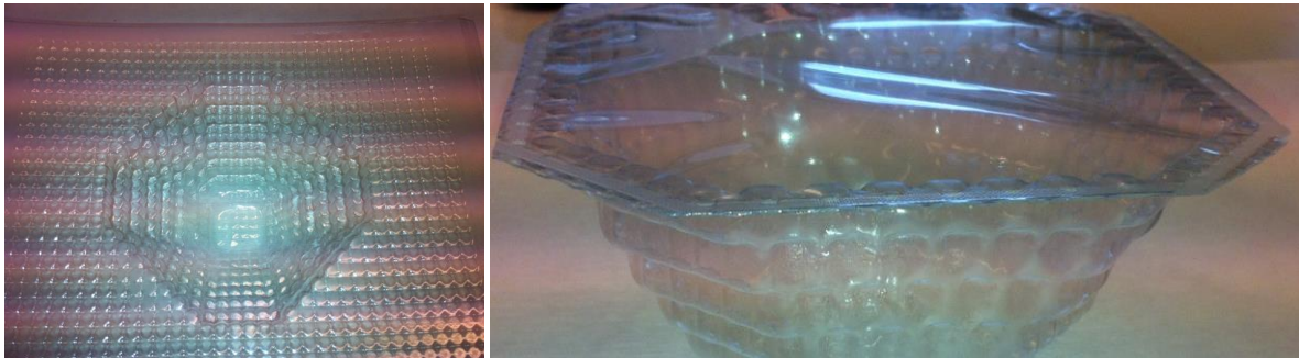
Figure 7 - Tray produced in a mould with 5 mm pins
