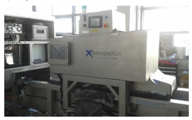
Figure 1. The X-ray sub-module in the PicknPack Line.
