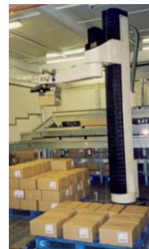
Figure 9 – Improvement measures to transfer boxes from conveyors to pallets
