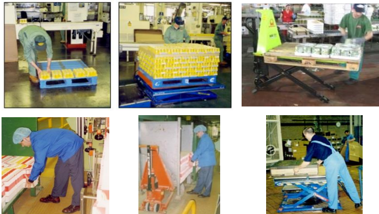
Figure 10 – Improvement measures to transfer boxes from conveyors to pallets
