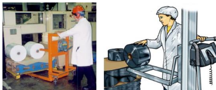
Figure 14 – Improvement measures to minimize rolls of packaging materials manipulation
