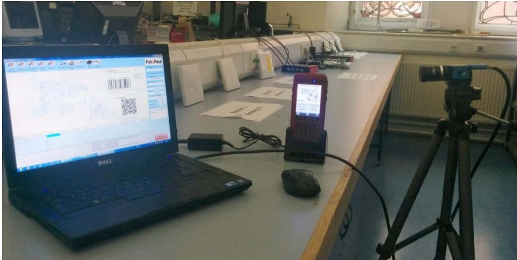
Figure 25 In-lab Test Bench of the RFID Traceability System
