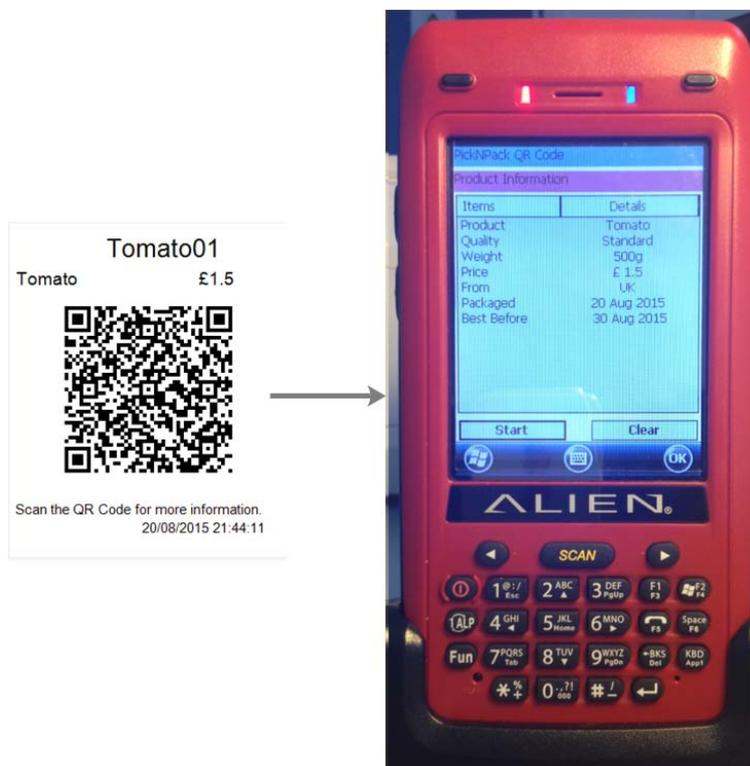
Figure 24 QR Code Decoding with Handheld Reader Application
