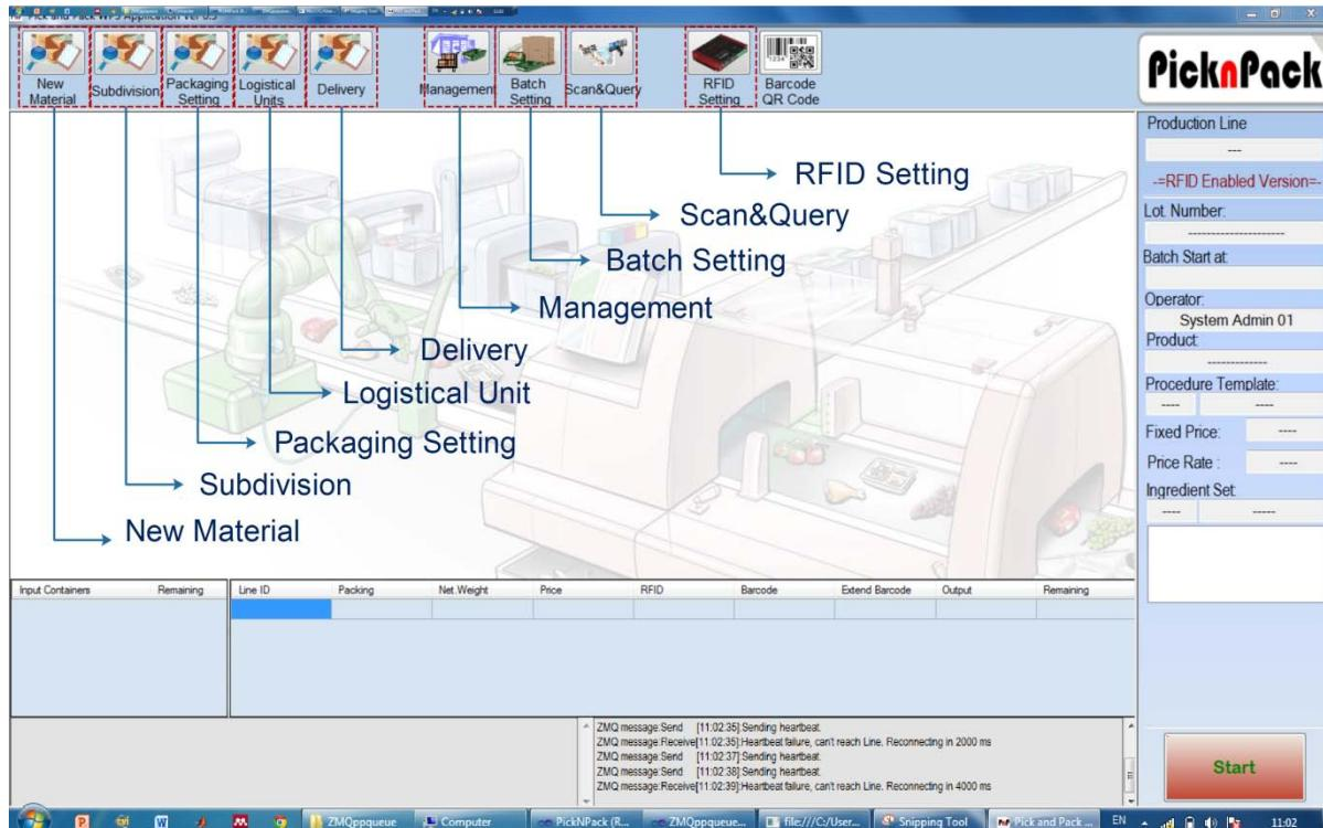
Figure 4 Main Interface of RFID Traceability System
