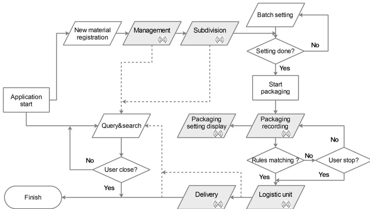
Figure 3 Process Model of the RFID Traceability System
