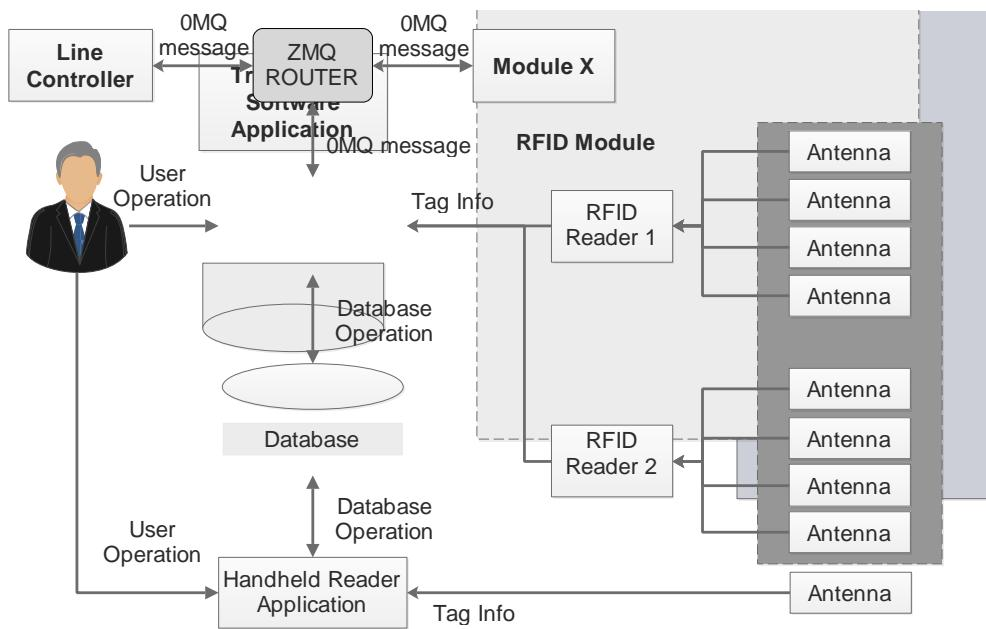
*Figure 1 Diagram of the Functional Modules*
