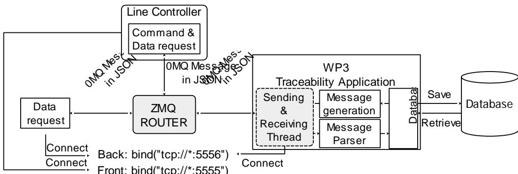
*Figure 2 ZMQ Interface for Data Request*
