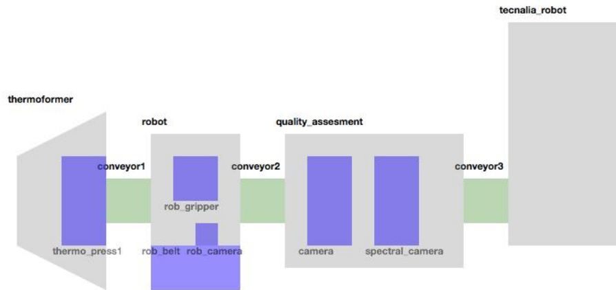
Figure 2: This shows a widget displaying an example geometry of a line with four modules and several devices. It also allows to select what is visualized by using the checkboxes at the top.
