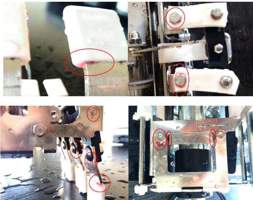
*Figure 40: Tomato gripper after Cleaning*
