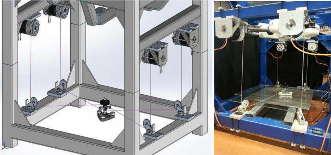
*Figure 13: Test bench for the test of cables, drums and winch behaviour*
