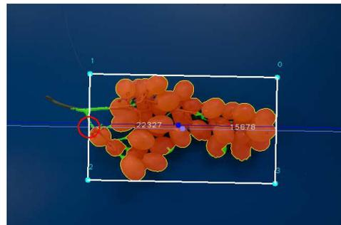
Figure 31 – An example of the detection of a grape vine. The preferred grasp is at the centre of the bounding box (light blue dot) and with the orientation of the bounding box (light blue line). The top of the bunch is marked with the red circle.
