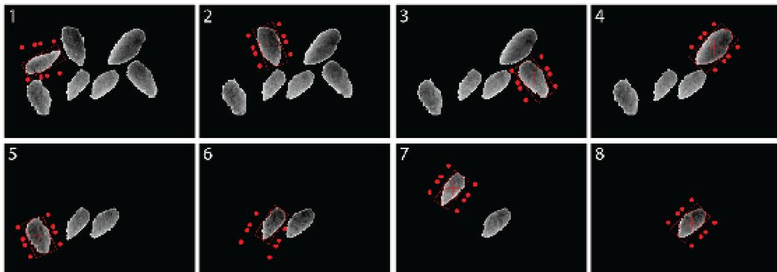
*Figure 30 – A sequence of grasps from left to right, top to bottom. 1, 3, and 6 are examples where the optimal grasp was not possible due to collisions and another position and orientation was proposed.*
