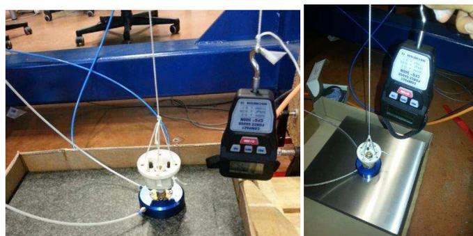
*Figure 9: Test of air bearings behaviour*
