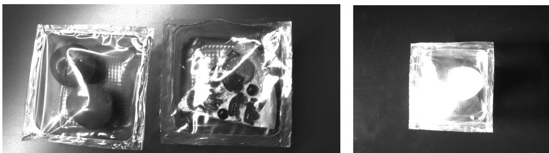
*Figure 33: Diffuse light vs selected light (high intensity, red)*
