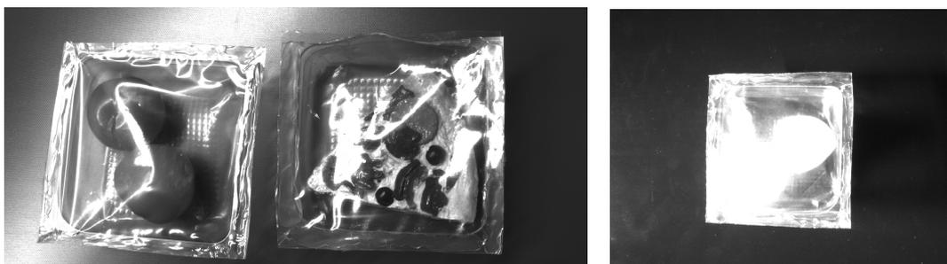
*Figure 33: Diffuse light vs selected light (high intensity, red)*
