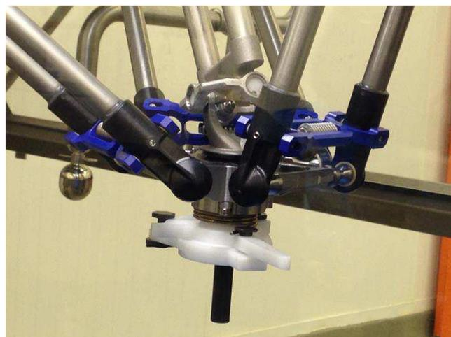
*Figure 19 Fast gripper changer*
