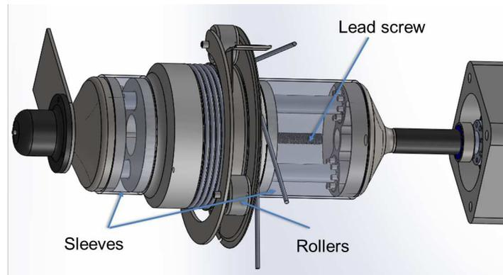
Figure 3: Detailed view of winch
