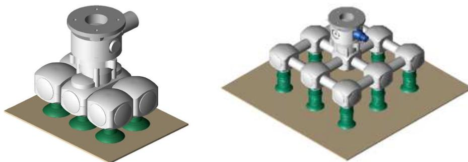
*Figure 23: Gripper design for packaging and other possible alternatives*
