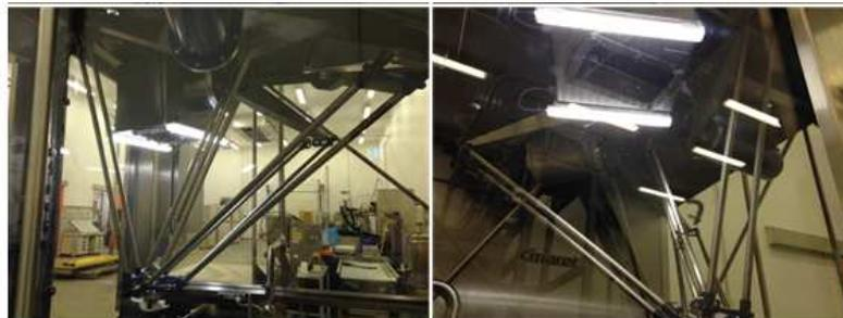
Figure 26 – The robot setup, including camera mounting and LED bars for illumination.
