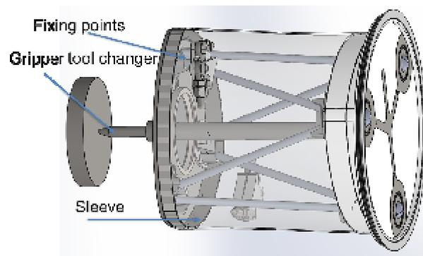
Figure 4: Detailed view of the platform
