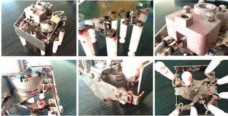
Figure 37: Chicken Gripper before Cleaning
