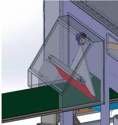
*Figure 36: Integrated vision system into the frame of the robot*
