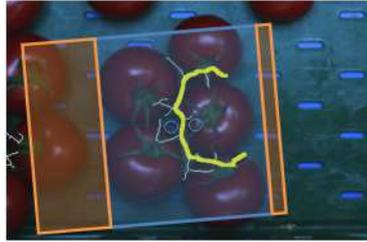
*Figure 28 – An illustration of the gripper placed on the vine. The blue circles form the pinch gripper. The small orange rectangle is the row of closed fingers and the larger orange rectangle is the row of open fingers. When opened, the fingers do not collide with other vine tomatoes.*
