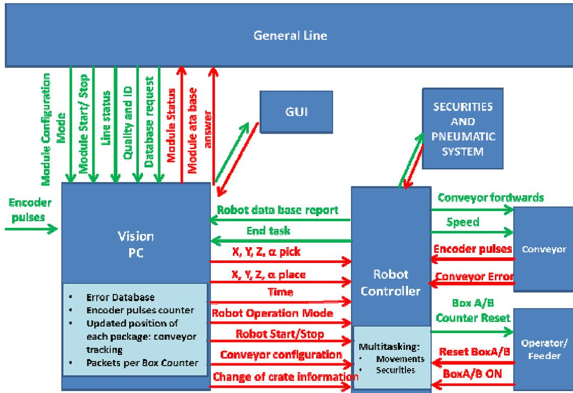
Figure 14: Internal and external communications of the cable robot module
