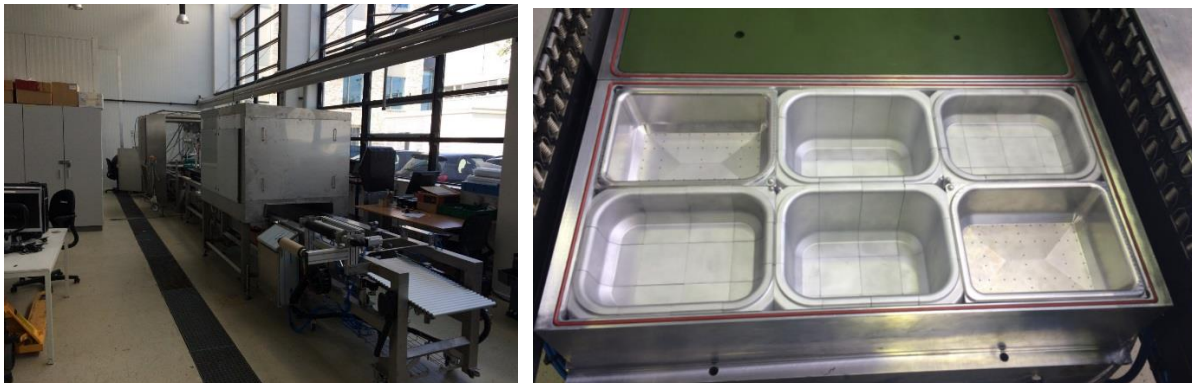
Figure 22 Photo of the integrated adaptive packaging line with brick moulds
