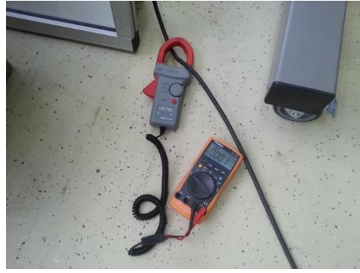
Figure 45 Efergy® E2 Classic three-phase units and amperometric clamps used for the experimental power measurements within the PicknPack line.
