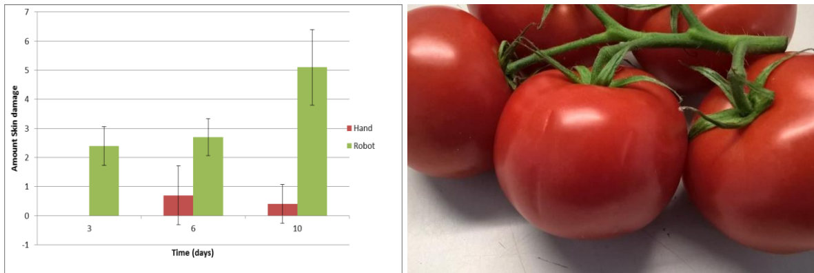
Figure 21: Left: Amount of mild skin damage on the tomatoes. Right: The fingers of the gripper cause mild skin damage.
