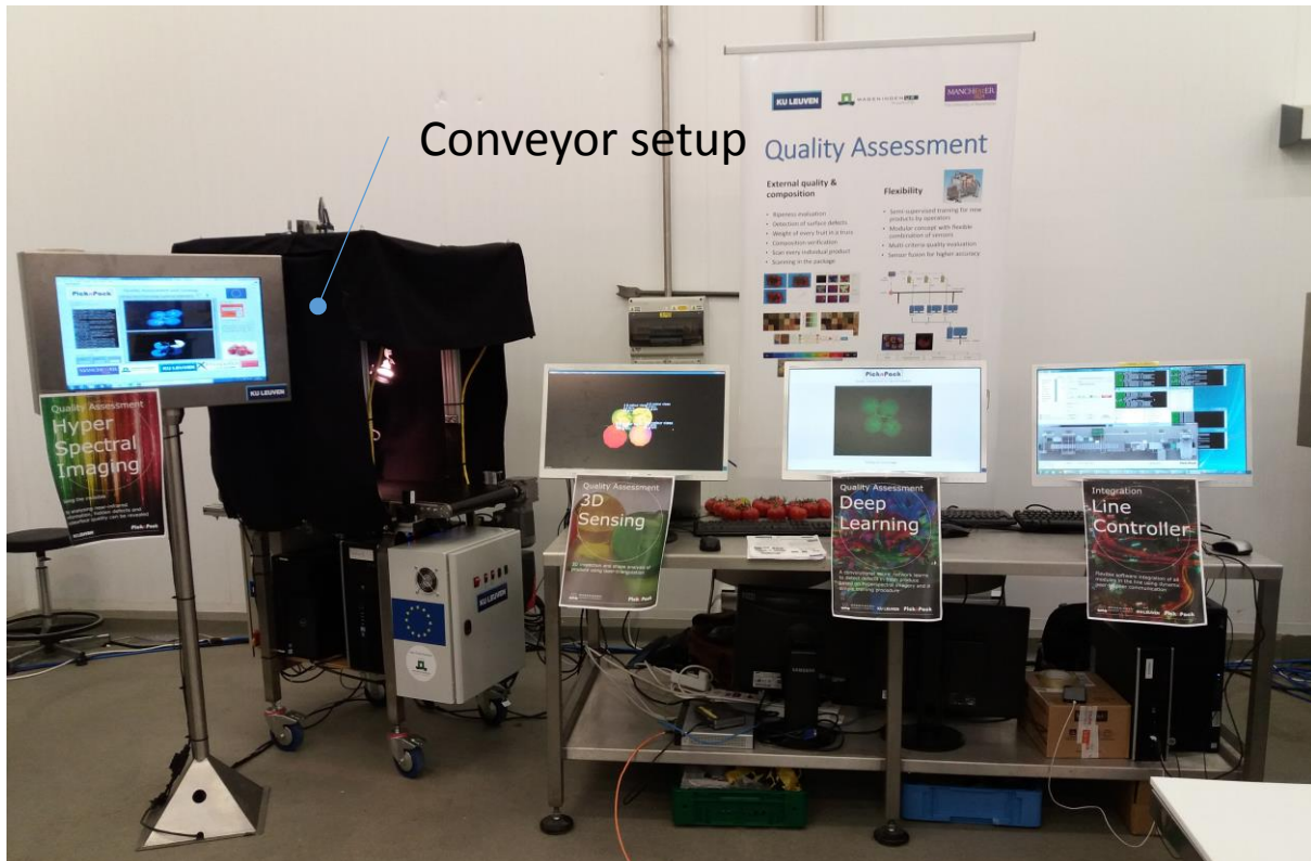
Figure 13 QAS setup, as demonstrated during the Holbeach demonstrations days. The conveyor setup contains the HSI and 3D sensors that are shielded from ambient illumination. The various screens surrounding the module display various aspects of the QAS module.
