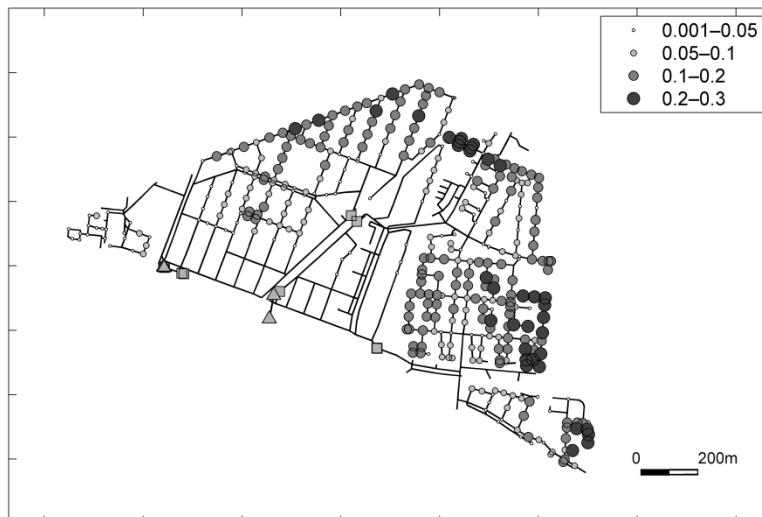
Figure 5.11: Example of spatial distribution of infection probability for children per year per manhole for a specific system state (i.e. Monte Carlo run) of 'Tuindorp' catchment.
