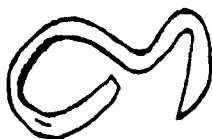
Fig. 8: A hoof pick can be easily made by bending a piece of round steel into the desired shape with one end flat and pointed.
