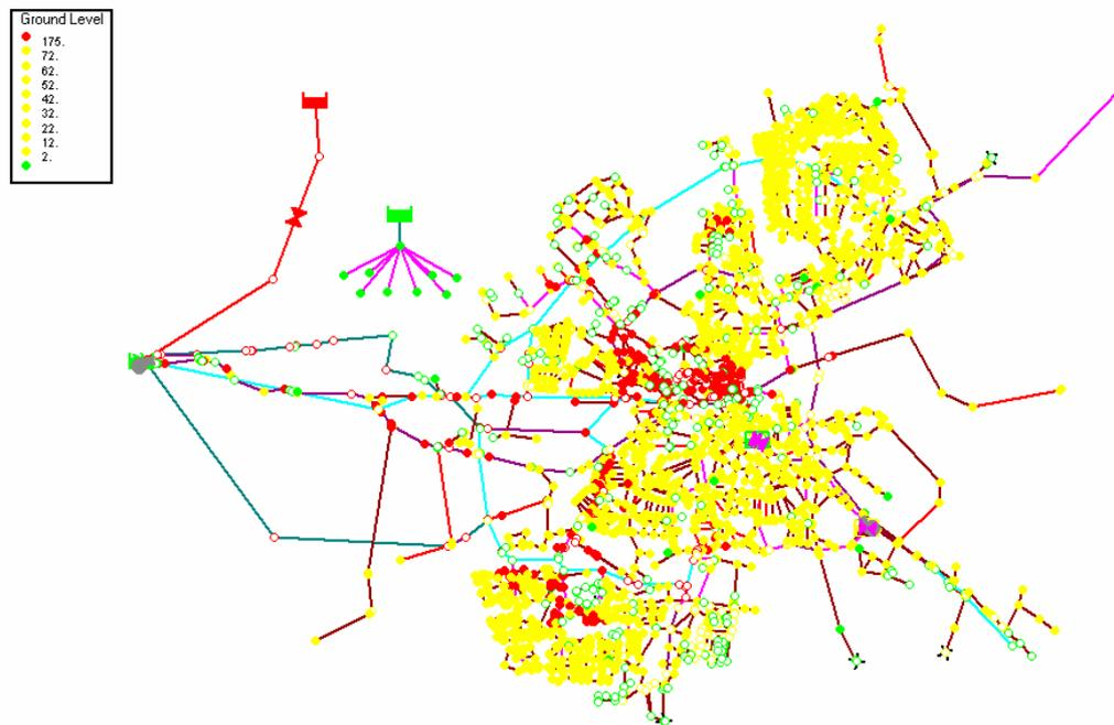
**Figure 2.3:** Calculated maximum concentrations when introducing a contaminant at the pumping station, reporting interval 30 minutes. The legend heading ground level should be replaced by concentration.
