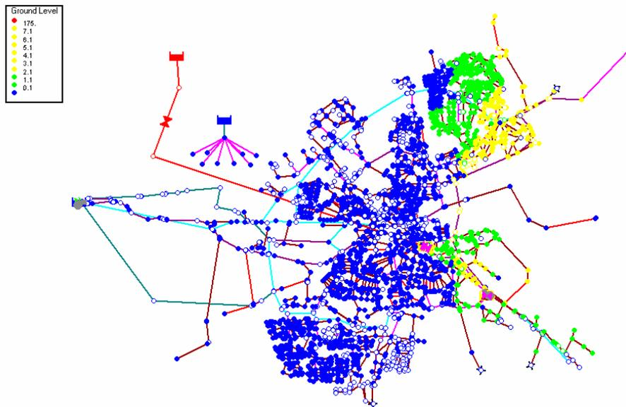
**Figure 2.9:** Calculated maximum concentrations when introducing a contaminant in the water tower, reporting interval 30 minutes. The legend heading ground level should be replaced by concentration.
