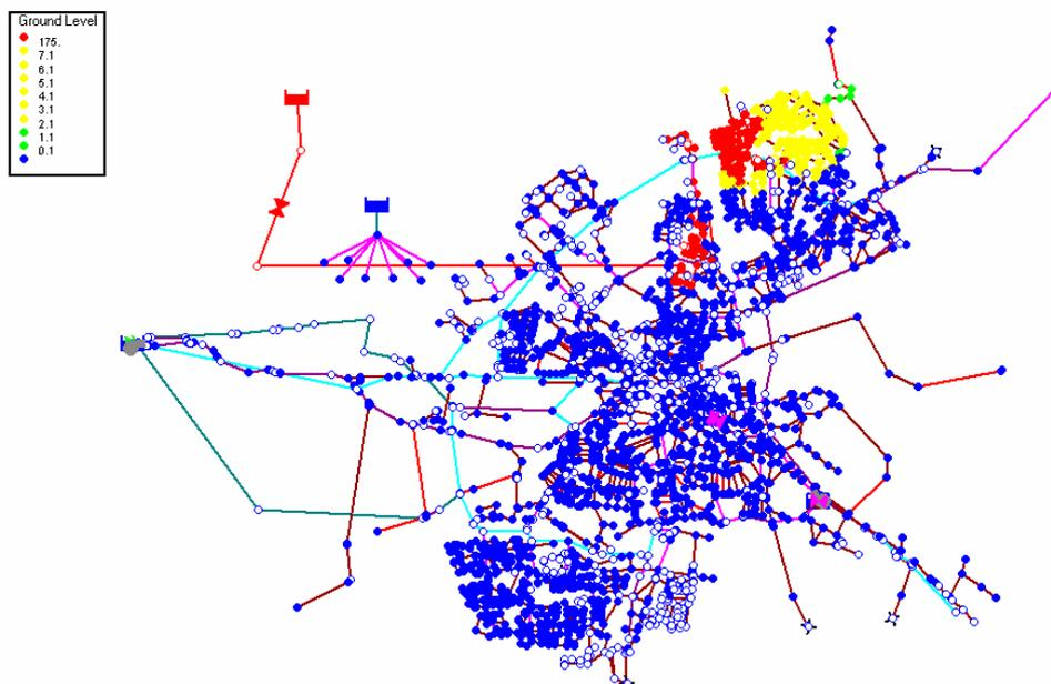
**Figure 2.8:** Calculated maximum concentrations when introducing a contaminant in a distribution pipe on the northern edge of the distribution area, reporting interval 30 minutes. The legend heading ground level should be replaced by concentration.
