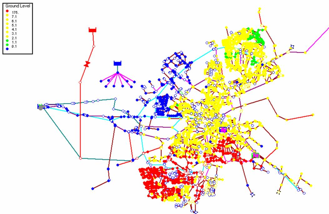
**Figure 2.6:** Calculated maximum concentrations when introducing a contaminant in a large supply main, reporting interval 30 minutes. The legend heading ground level should be replaced by concentration.
