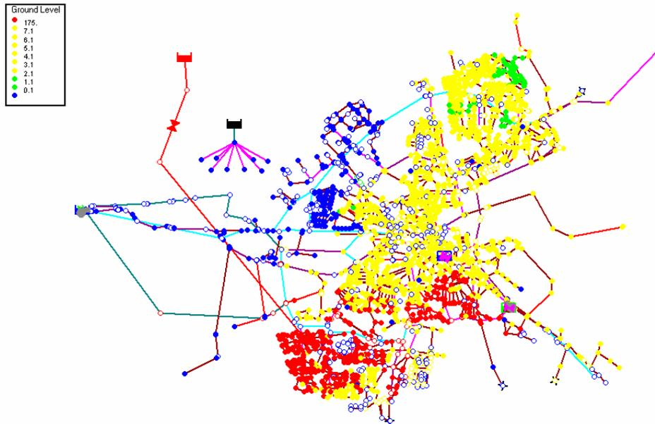
**Figure 2.7:** Calculated maximum concentrations when introducing a contaminant in a distribution pipe on the southern edge of the distribution area, reporting interval 30 minutes. The legend heading ground level should be replaced by concentration.
