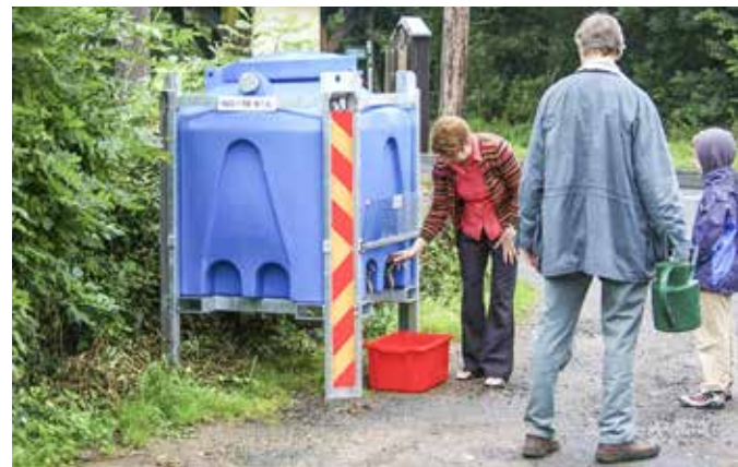
Mobiele drinkwatertank in Gloucestershire
