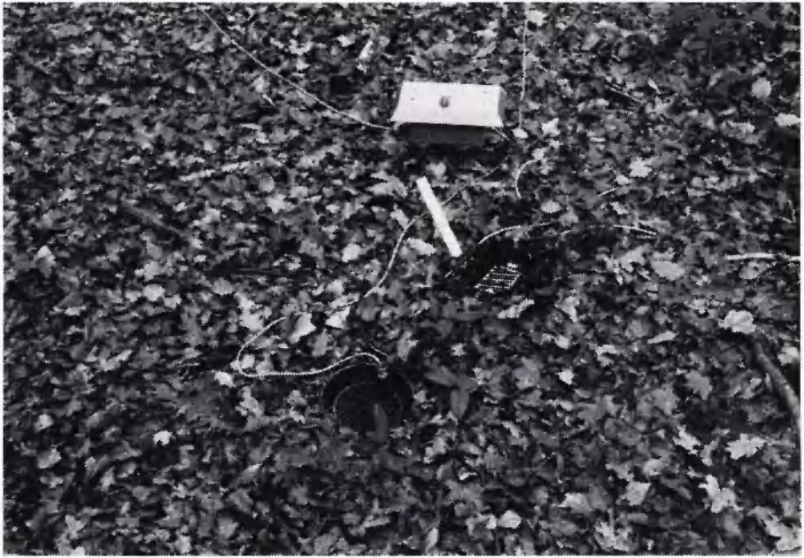
Photo 3. The same as photo 2, but now the sensor for measuring surface humidity has been uncovered, and the perspex roof has been taken away to show the entrance of the (asymmetrical) funnel of the pitfall with a gitter to keep out litter and animals such as mice, shrews, frogs and toads.
