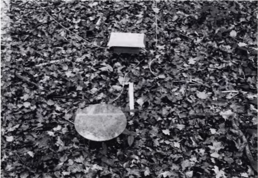
Photo 2. A single time-sorting pitfall 'in situ' (covered with a transparent perspex roof). In the background the electronic unit for converting the primary signals concerning surface temperature and humidity.
