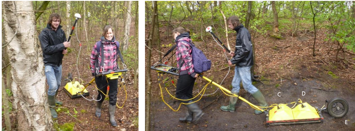
Figure 18 The pulse EKKO pro GPR measurement device as used in this research. A: Measurement device that record and display the signal. B: GPS device. C: Transmitter (250 MHz). D: Receiver. E: Odometer: measuring distance. Source: own pictures.
