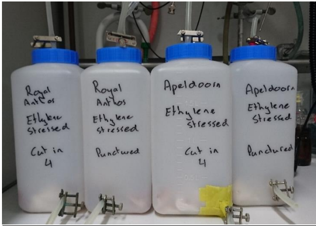
Appendix 2; Air-tight containers for ethylene stressing of both Royal Anthos and Apeldoorn tulip biomass
