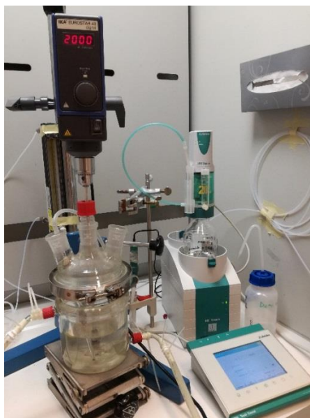
Figure 5. Heterogeneous oxidation set up 2 for the reactions conducted with catalyst supported on AC.
