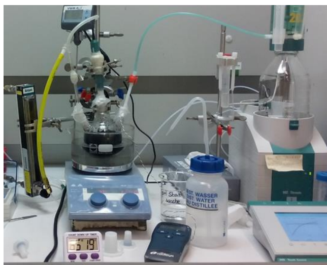
Figure 4. Heterogeneous oxidation set up 1 for the reactions conducted with catalyst supported on AC.
