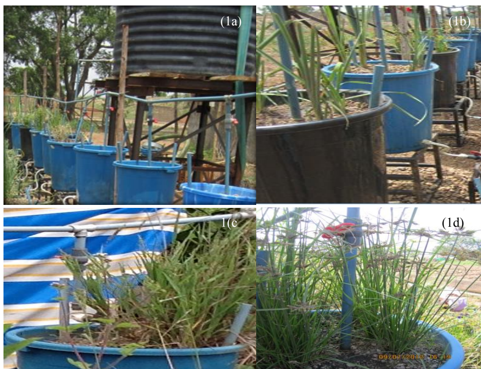
Fig.4.1. (a) Experimental set up, (b) the macrophytes at start-up, (c) C. dactylon five months after planting and (d) C. alternifolius five months after planting.
