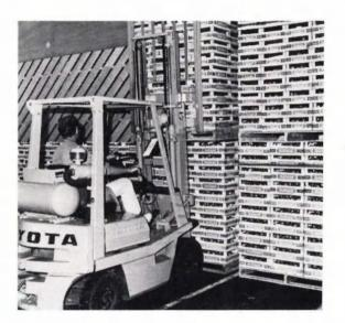
Precooling of tomatoes by means of a pressure wall
