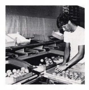
After sorting for colour and size the trays are being filled up till the correct weight <u>Quality sorting</u> is generally done by hand immediately after size sorting, and is done on the tables or conveyor belts of the sizer. Ribbed tomatoes, > 67mm, are also sorted by hand, at the same moment as the size grading.
