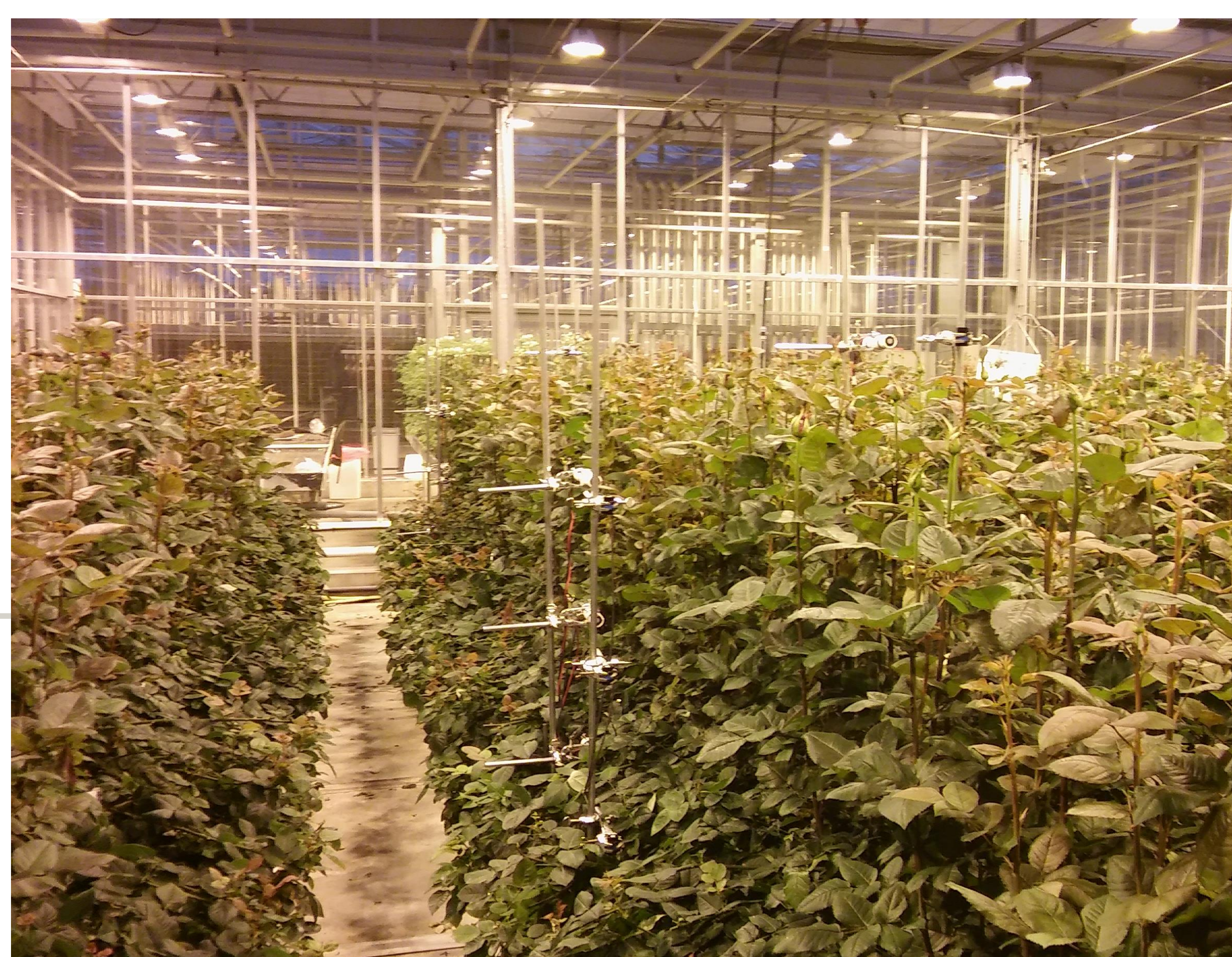
Figure 2. Profile of PAR sensors in a rose greenhouse. Next to PAR, also temperature and relative humidity are measured.
