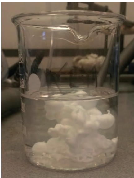
EXAMPLE OF POLYMER PRECIPITATE IN ACETONE
