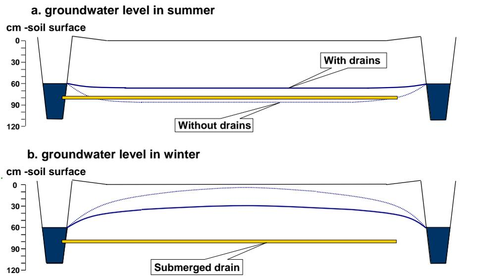
**Fig. 1: Reduction of peat oxidation and subsidence and CO<sub>2</sub>-emissions by raising groundwater levels with infiltration via submerged drains in summer level. In wet periods the submerged drains will function as drainage.**
